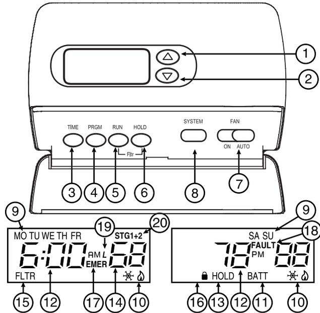
Figure 6 – Thermostat display, buttons and switches
