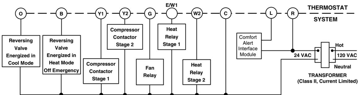
Figure 5. Typical wiring diagram for single transformer multi-stage systems
