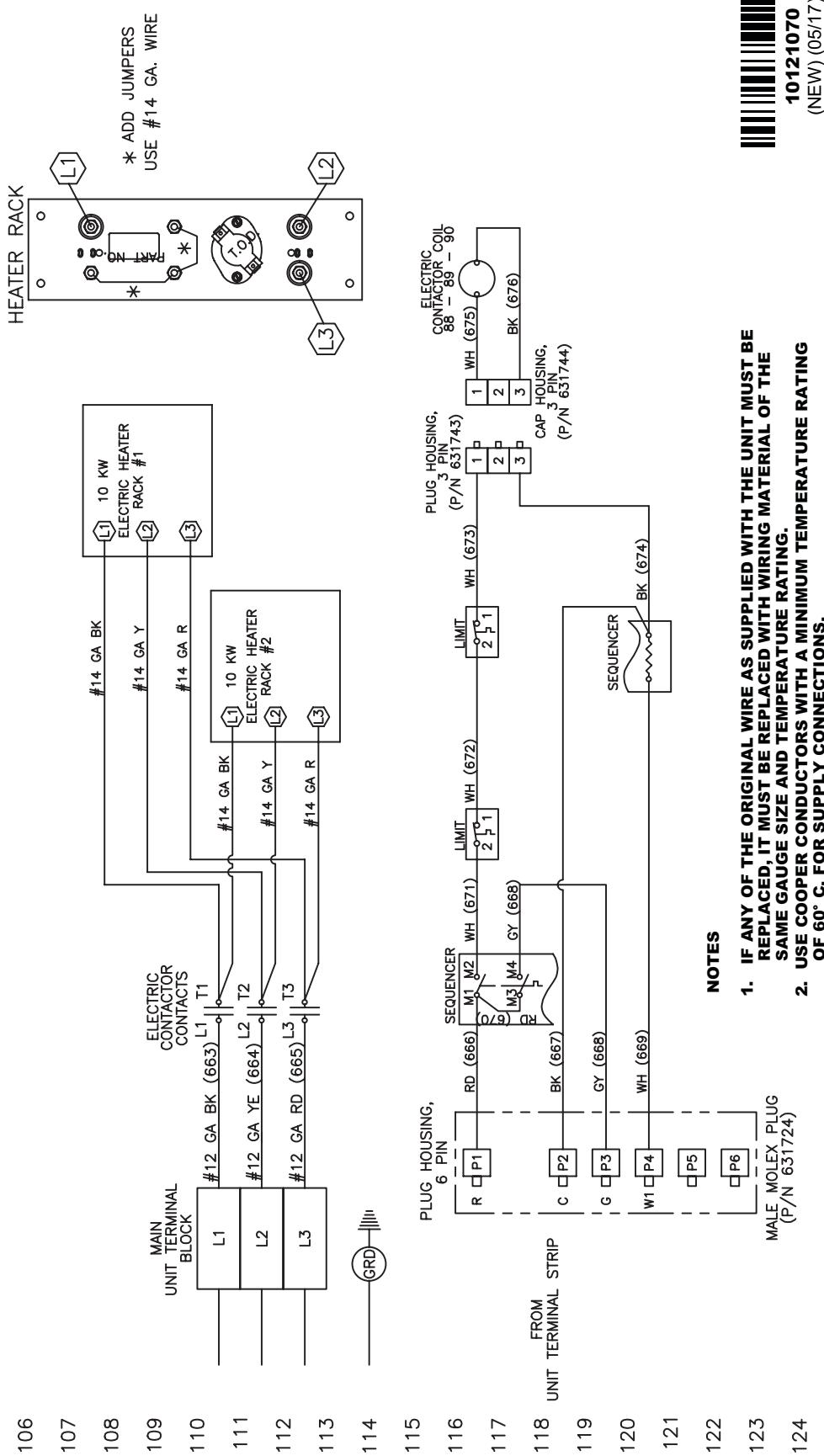
Figure 19. W.D. for 20 kW, 575 V, 3-Phase
