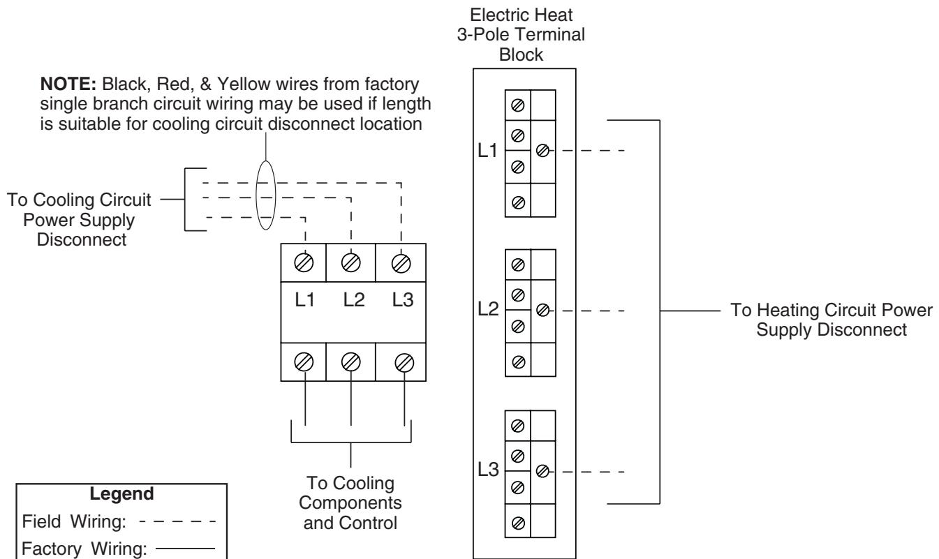
**Figure 13. Single & Dual Power Supply Connections**
