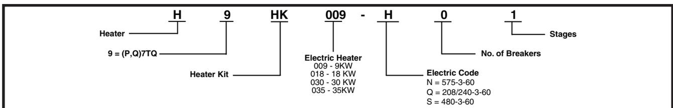
Figure 1. Heater Kit Identification Code
