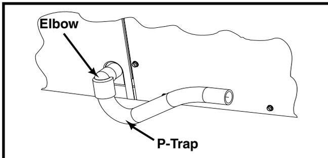
Figure 6. Drain Trap
