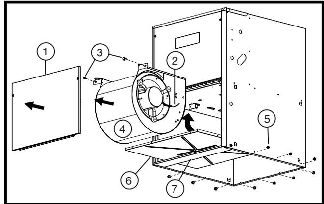
Figure 16. Bottom Panel Removal
