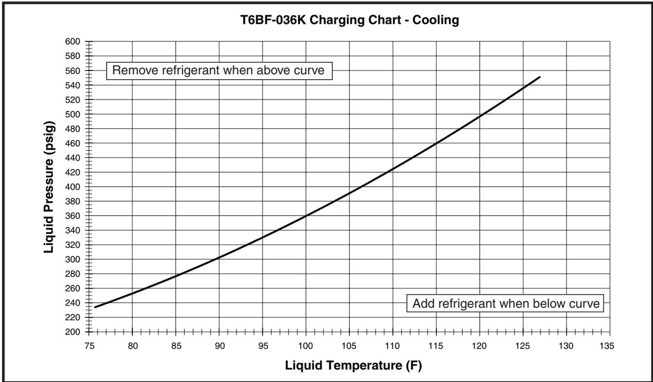
**Figure 7. Charging Chart for 3 Ton Models
