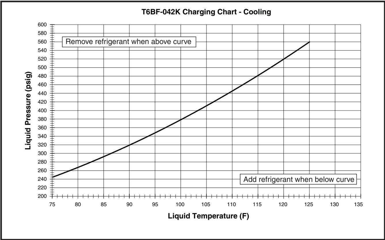
**Figure 8. Charging Chart for 3.5 Ton Models
