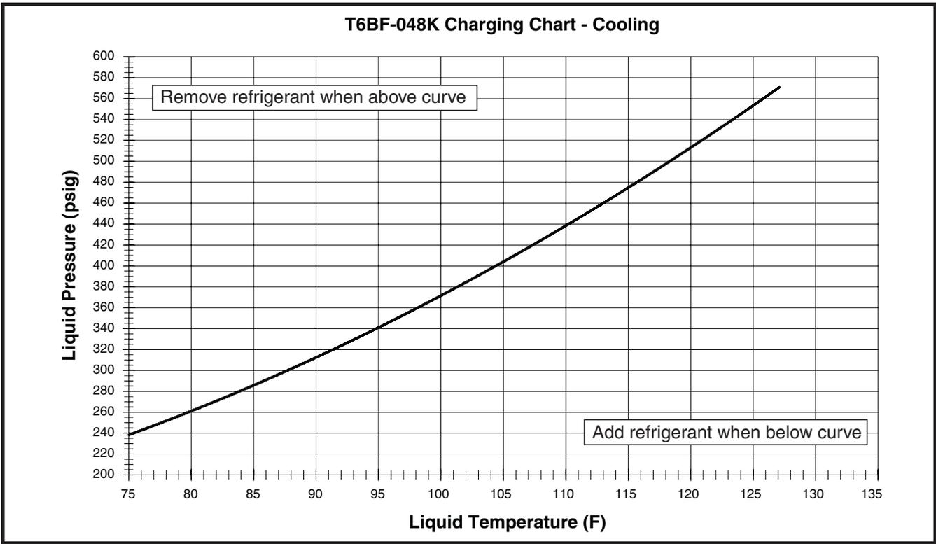
**Figure 9. Charging Chart for 4 Ton Models
