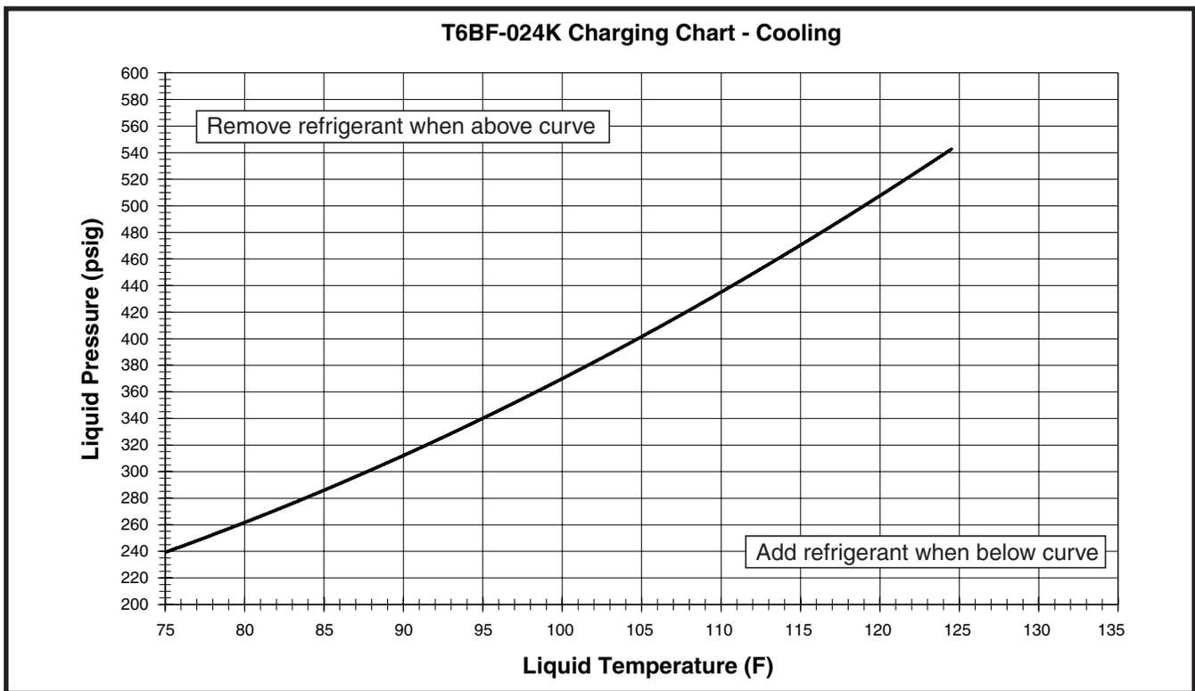
Figure 5. Charging Chart for 2 Ton Models
