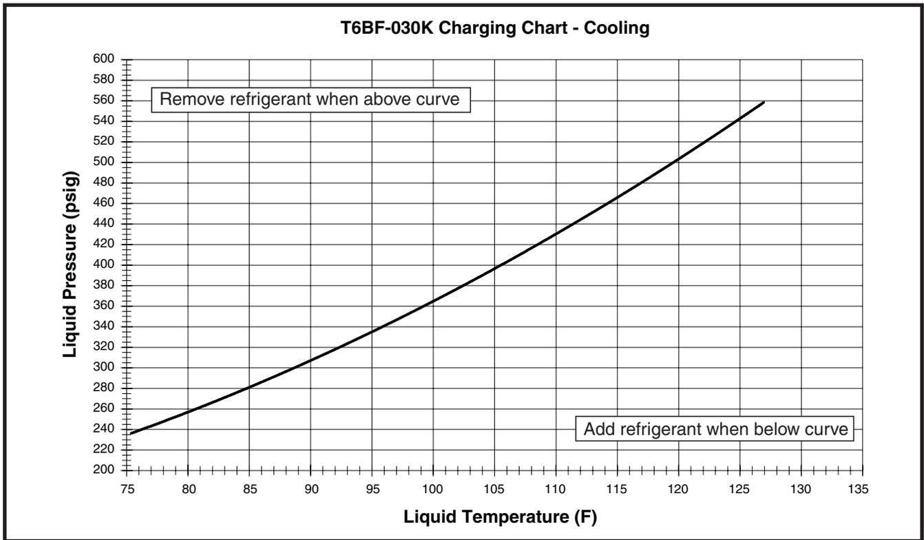
**Figure 6. Charging Chart for 2.5 Ton Models
