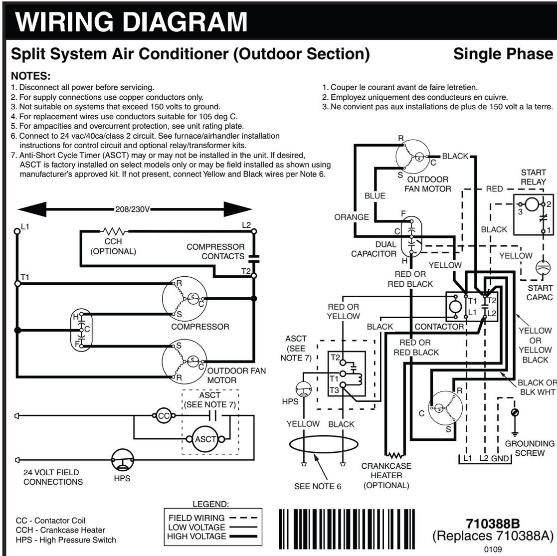
**Figure 4. Wiring Diagram for 1.5 - 4 Ton Models (without CoreSense™)**
