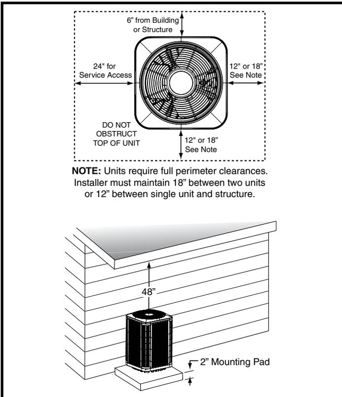
**Figure 1. Clearance Requirements**
