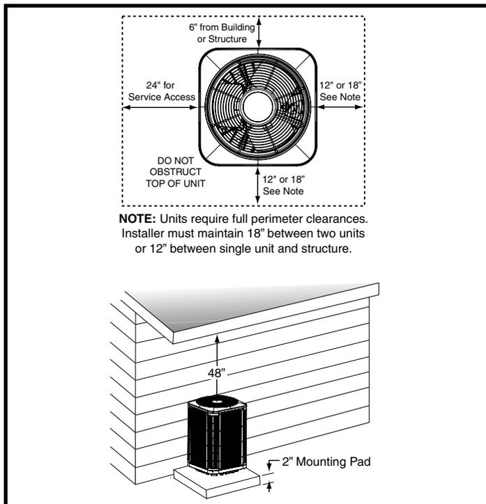
Figure 1. Clearance Requirements
