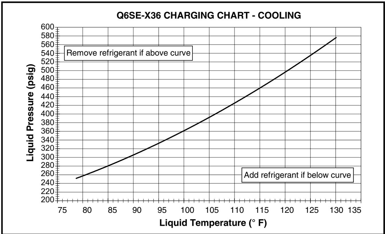
Figure 12. Charging Chart for 3 Ton Units
