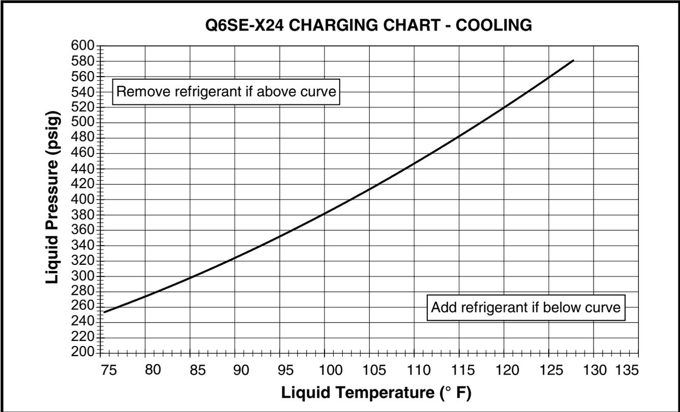
Figure 10. Charging Chart for 2 Ton Units
