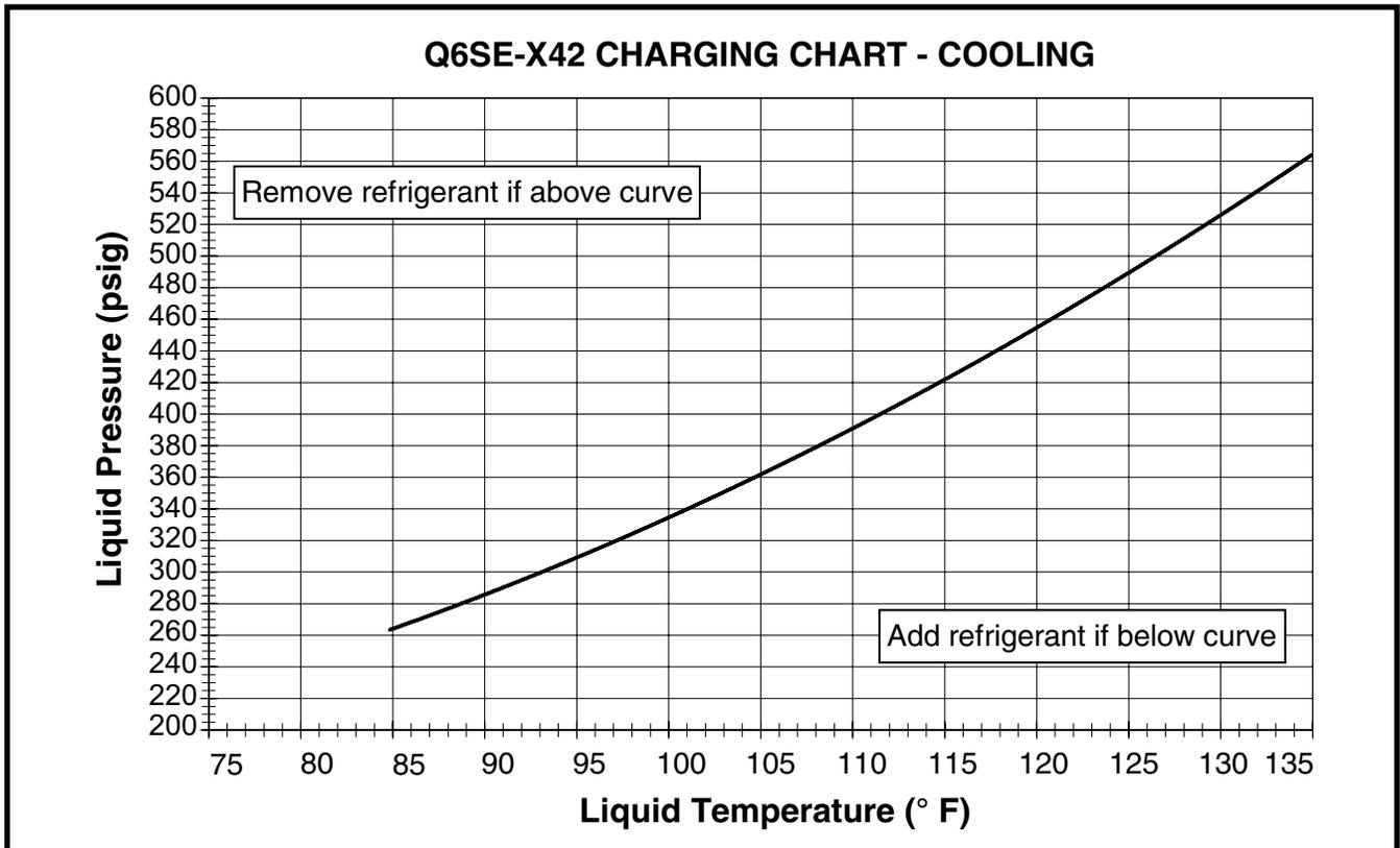
Figure 13. Charging Chart for 3.5 Ton Units
