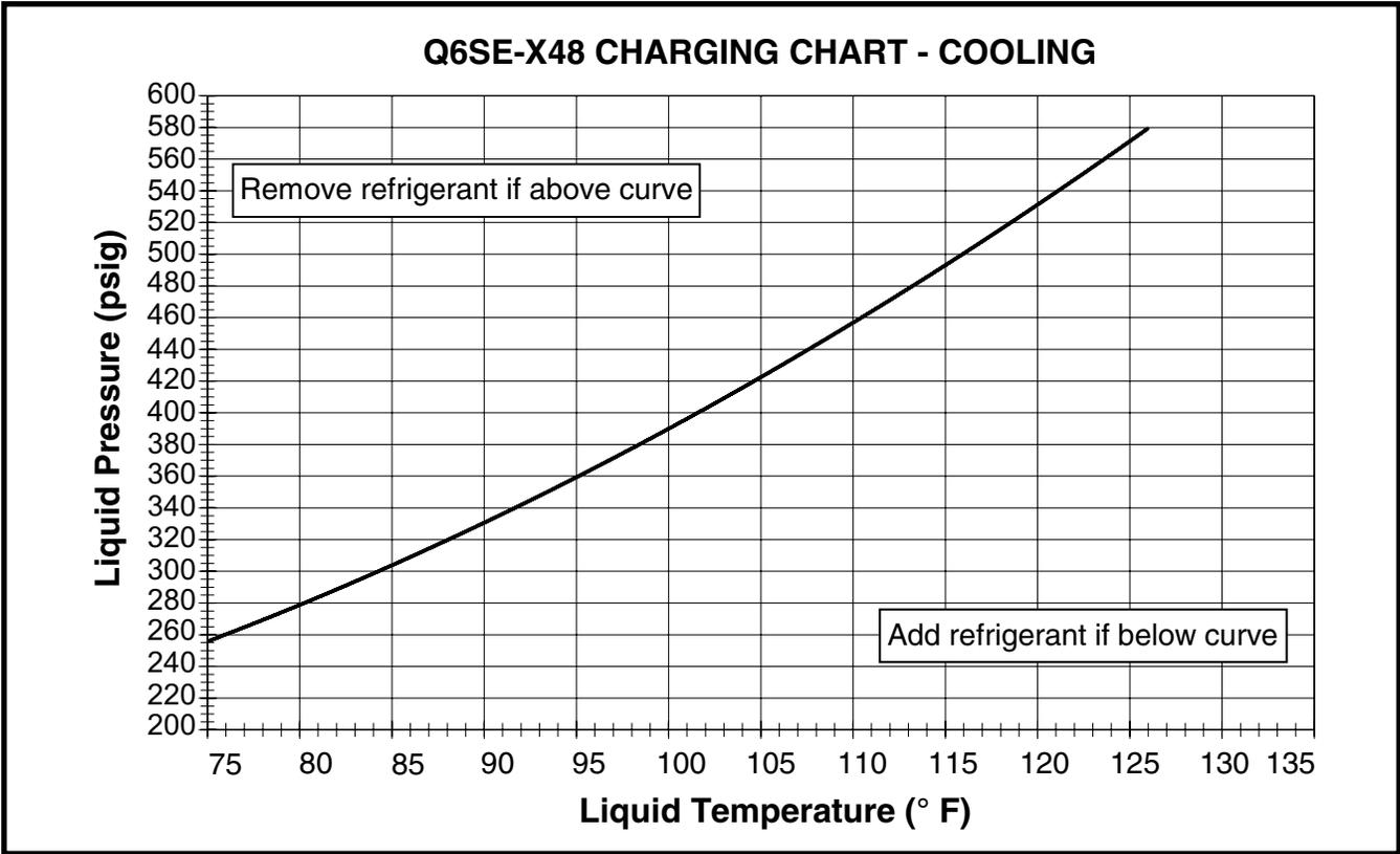
Figure 14. Charging Chart for 4 Ton Units
