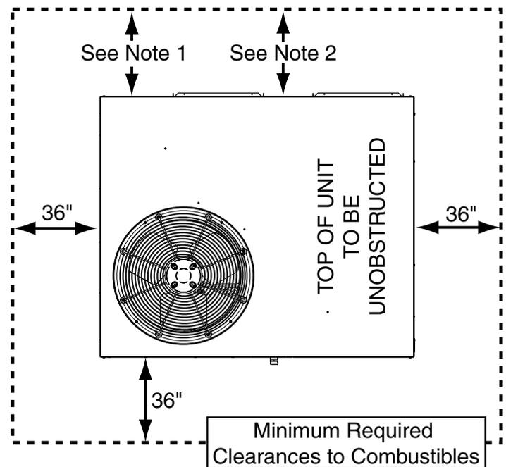
**NOTE 1:** 6" When coil is present on duct side.
