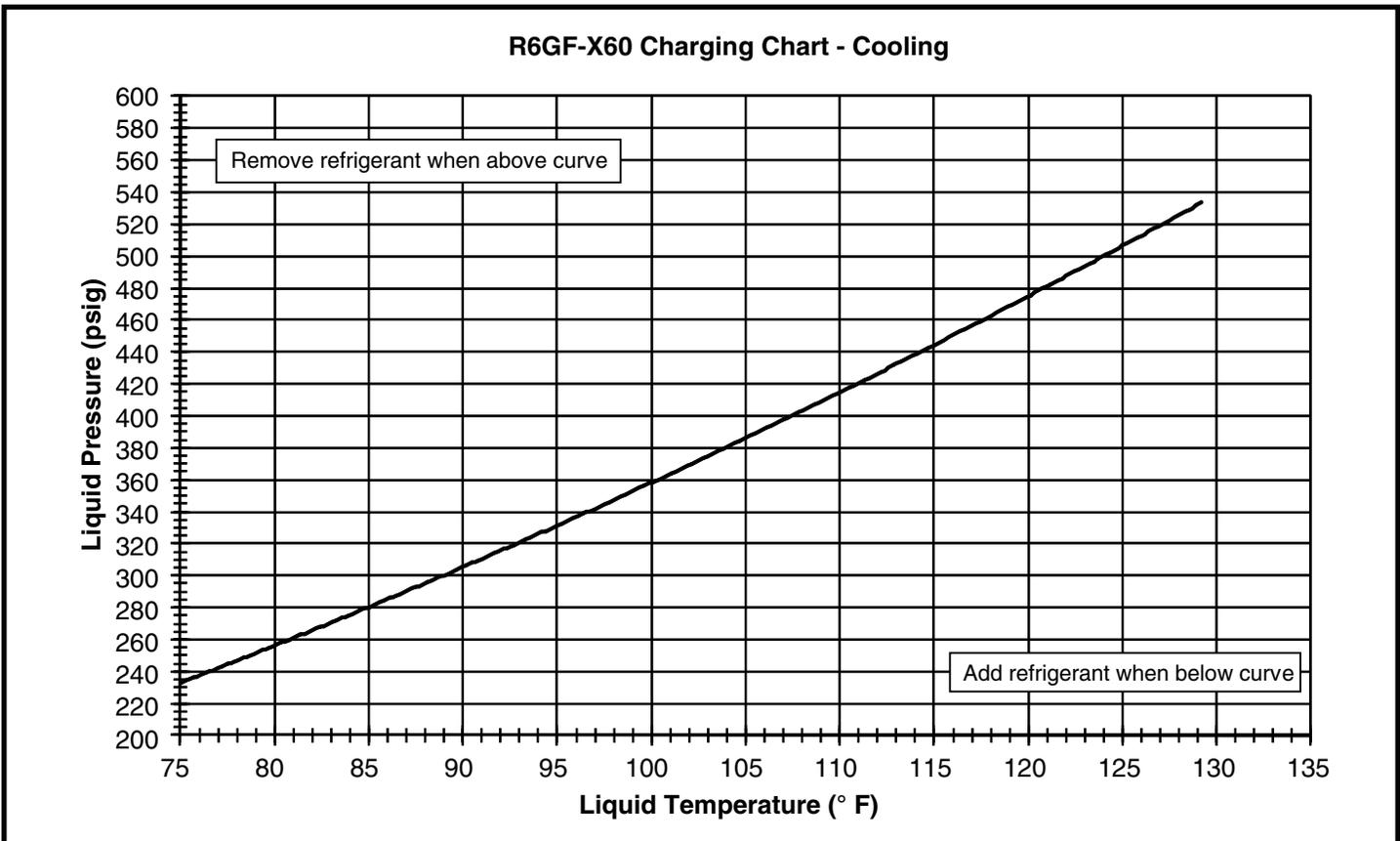
**Figure 18. Charging Chart for 5 Ton Units**
