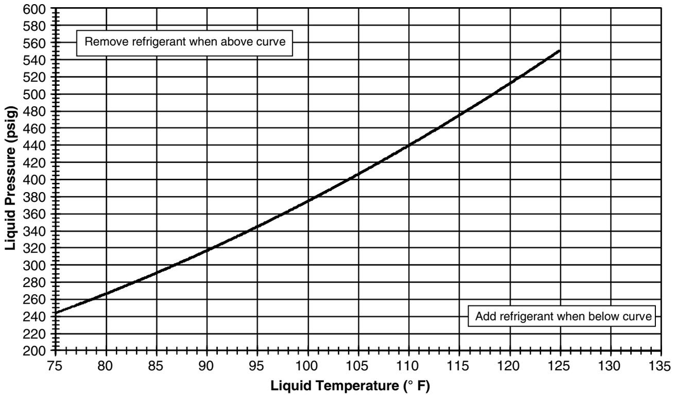
Figure 15. Charging Chart for 2 Ton Units
