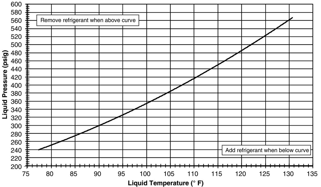
Figure 16. Charging Chart for 3 Ton Units
