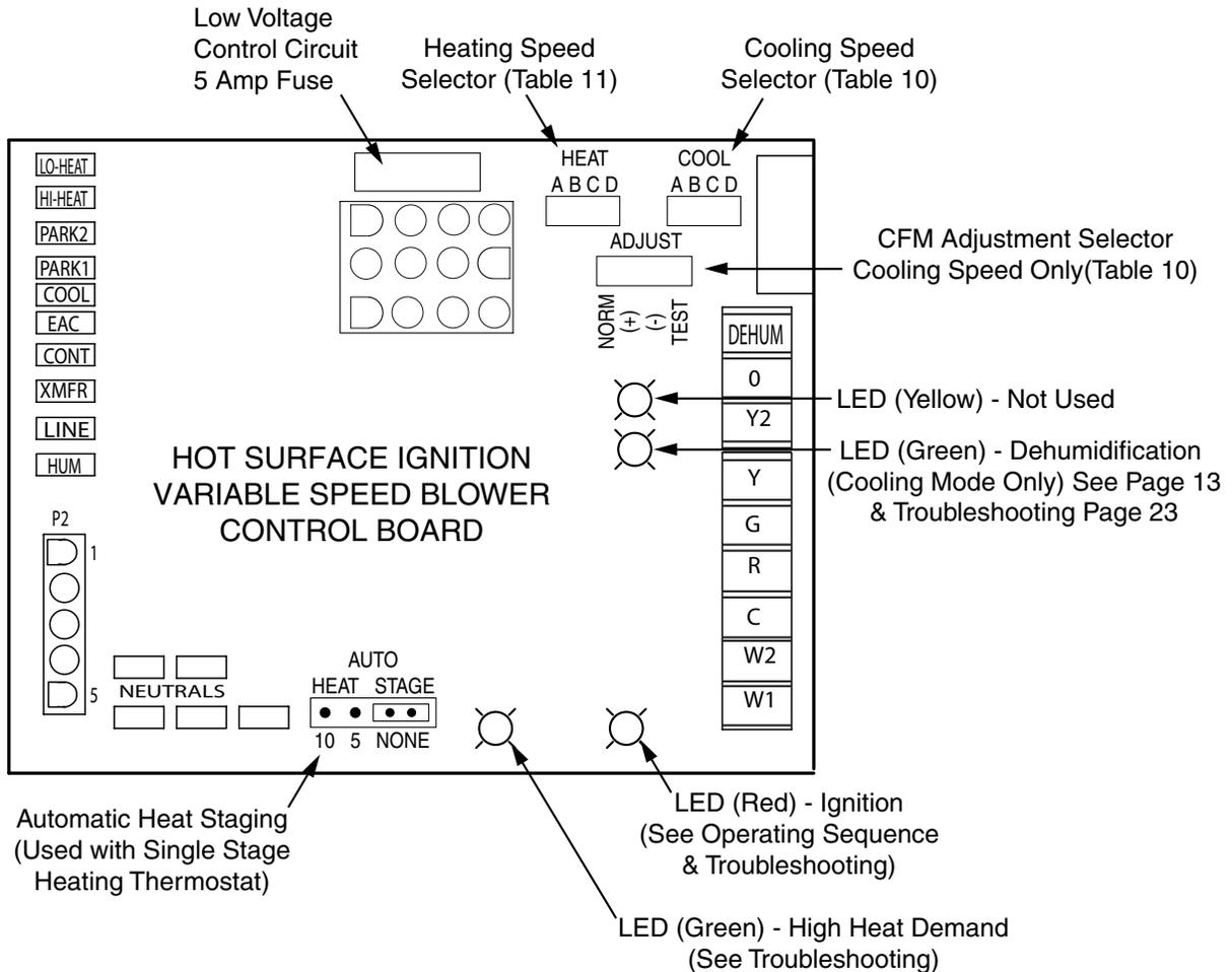
**Figure 12. Two-Stage, Hot Surface Ignition & Blower Control Board**
