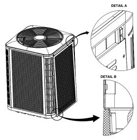
Figure 5. Panel Installation
