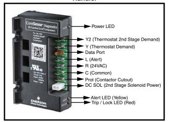
Figure 3. CoreSense™ Diagnostics Module
