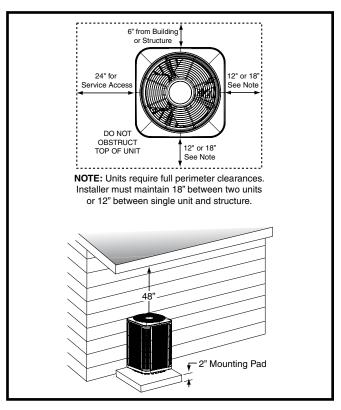
Figure 1. Clearance Requirements
