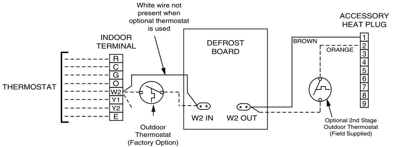
**Figure 12. Typical Thermostat Connections**
