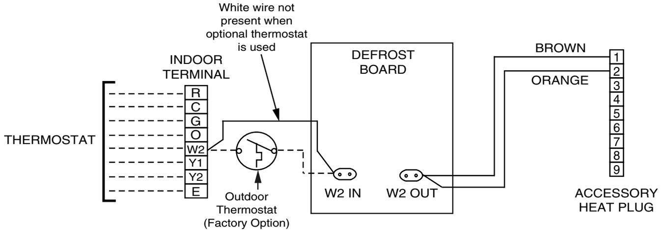
**Typical Wiring (Field Supplied) for 1-Stage Cool, 2 Stage Electric Heat**
