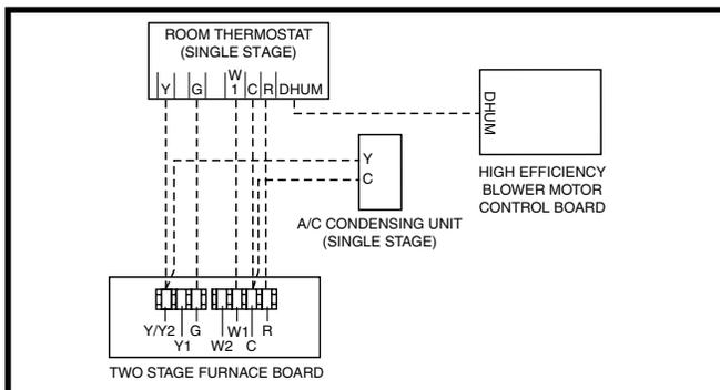
Figure 15. Wiring Configuration 1
