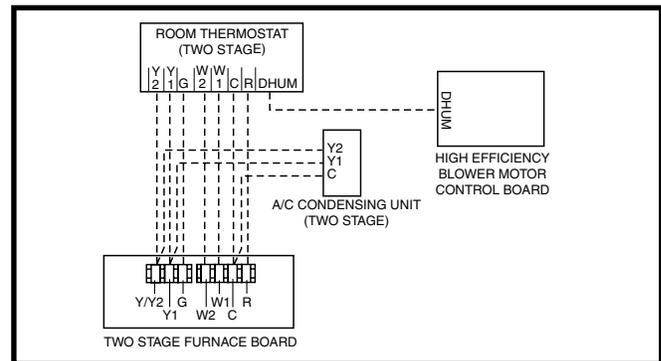
Figure 17. Wiring Configuration 3
