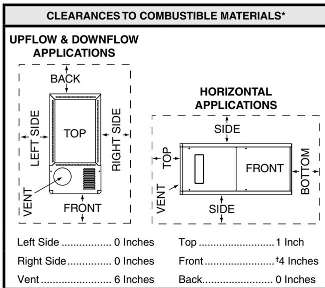
\*Allow 24 in. minimum clearance for servicing. Recommended clearance is 36 in.
