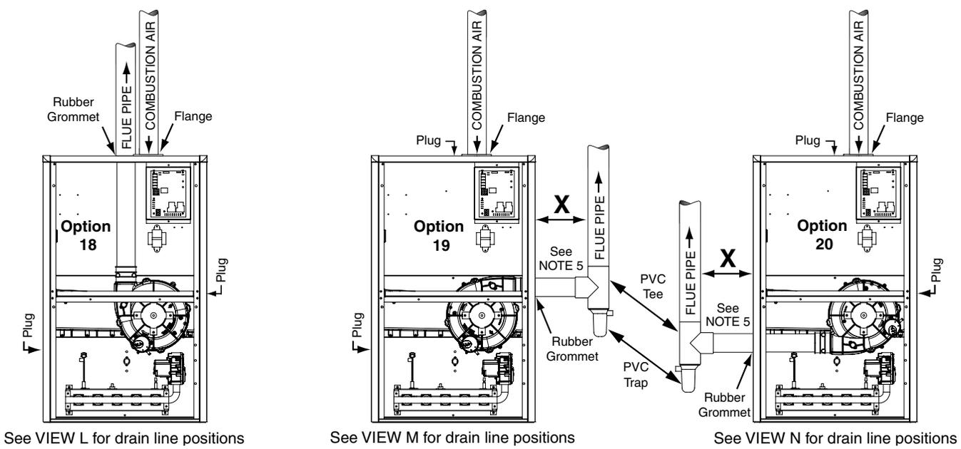
**Figure 38. Venting Options for Downflow Installations (\*SL Series)**
