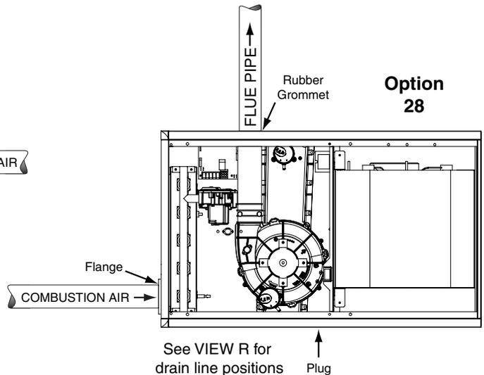
**Figure 41. Venting Options for Horizontal Installations (\*SD Series)**
