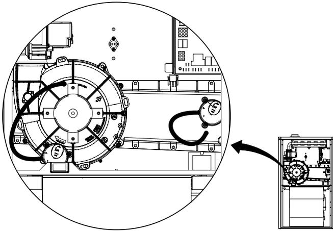
**Figure 15. Pressure Switch Tubing for Upflow Furnaces**
