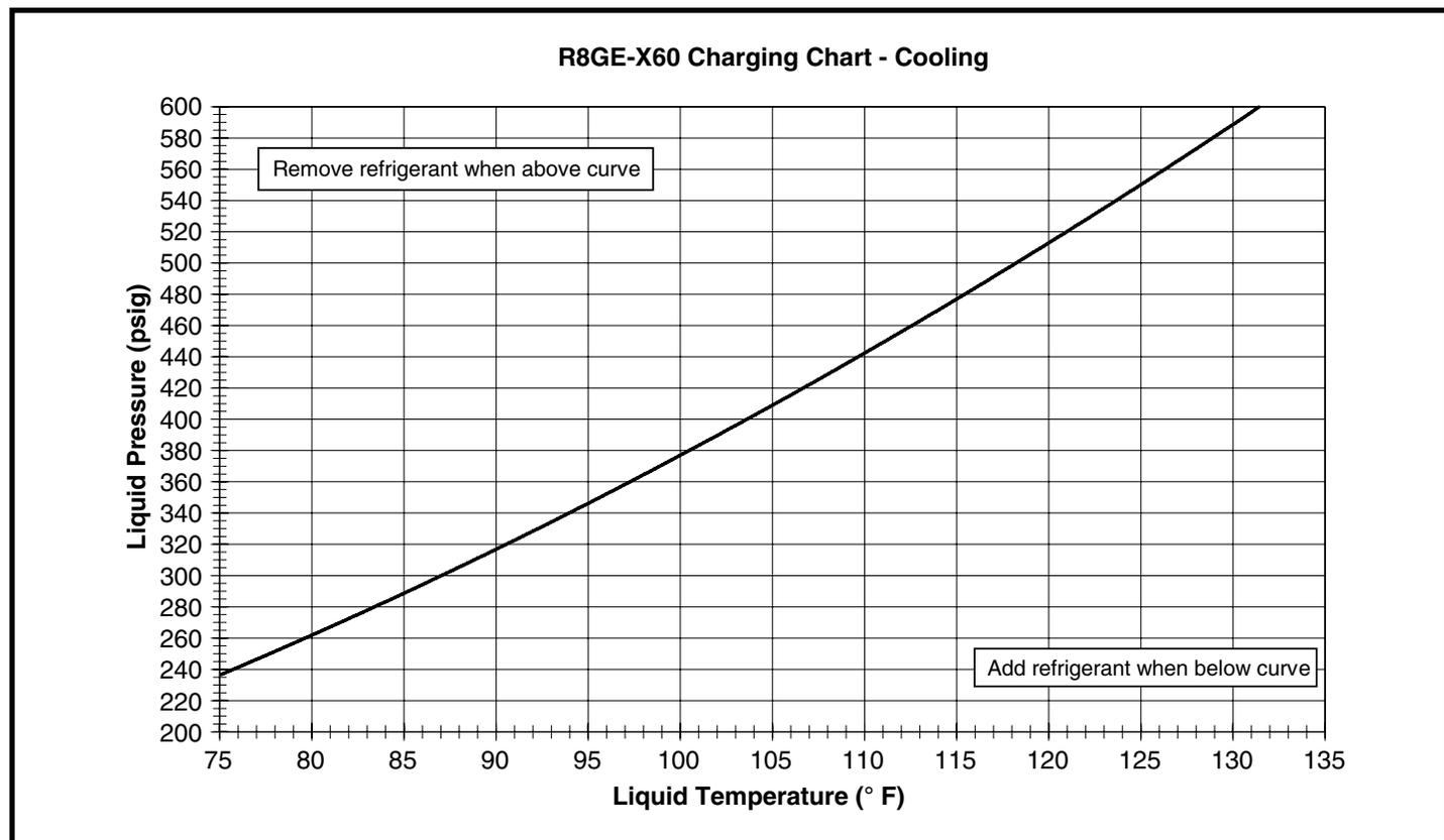
Figure 12. Charging Chart for 5 Ton Models
