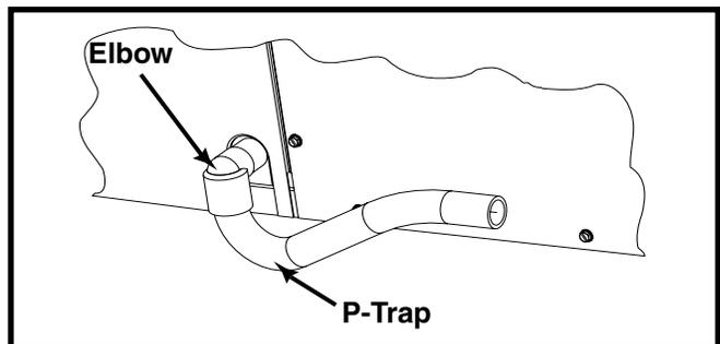
**Figure 6. Drain Trap**
