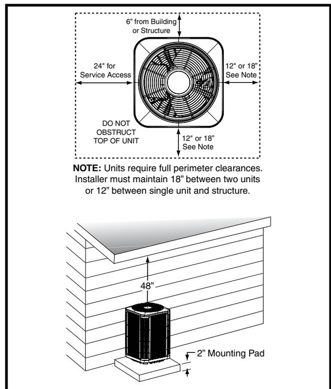
**Figure 1. Clearance Requirements**
