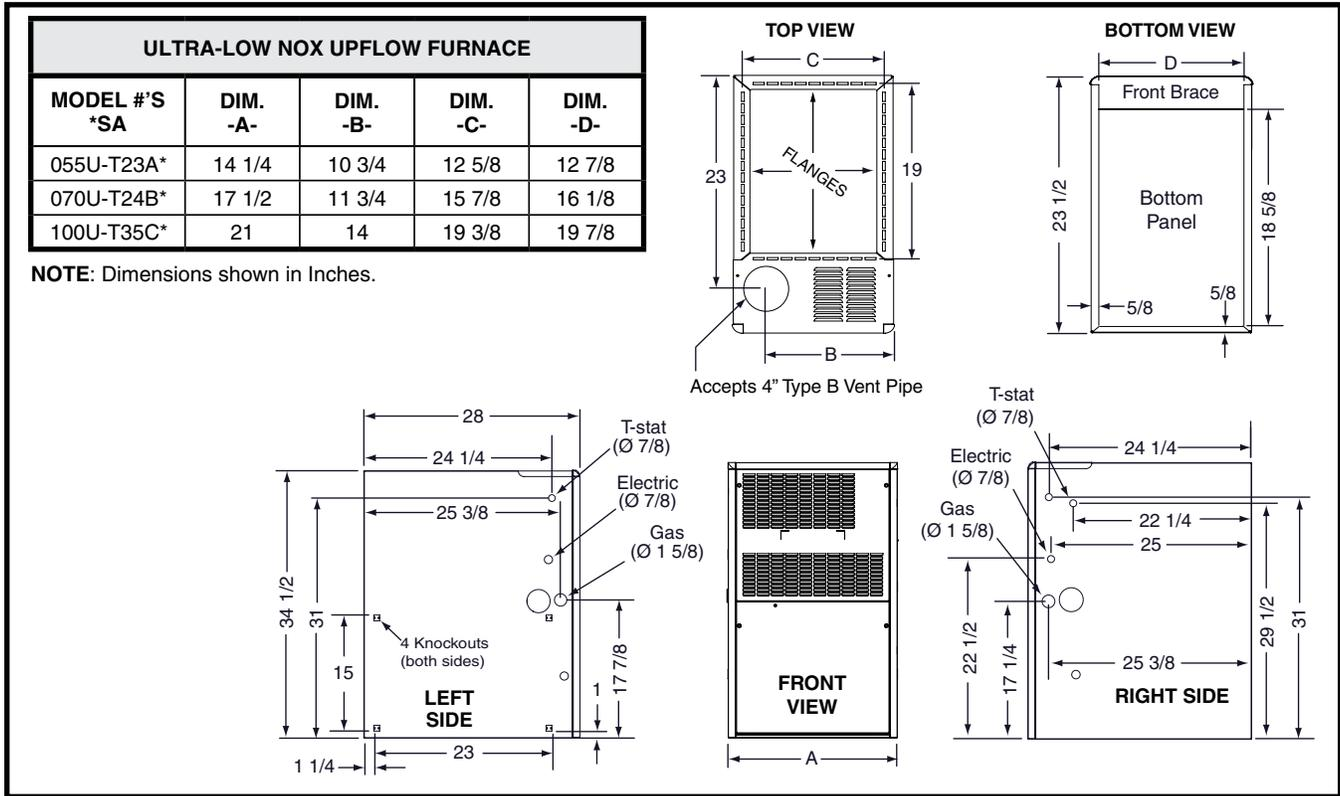
**Figure 18. Furnace Dimensions**
