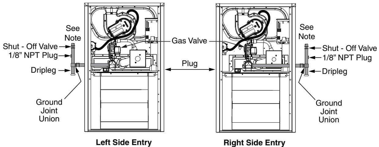
**NOTE:** Some utilities require Shut - Off Valve to be 4 - 5 feet above floor.
