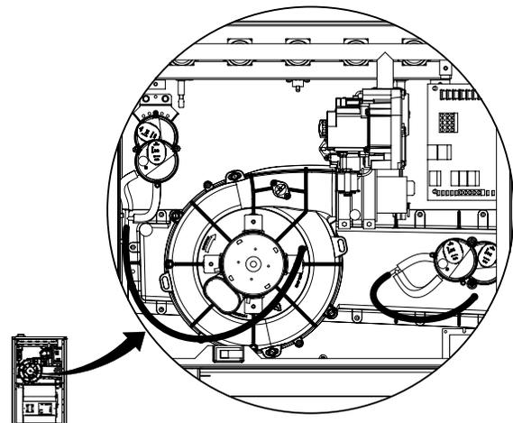
**Figure 13. Pressure Switch Tubing for \*TC Upflow / Horizontal Furnaces**
