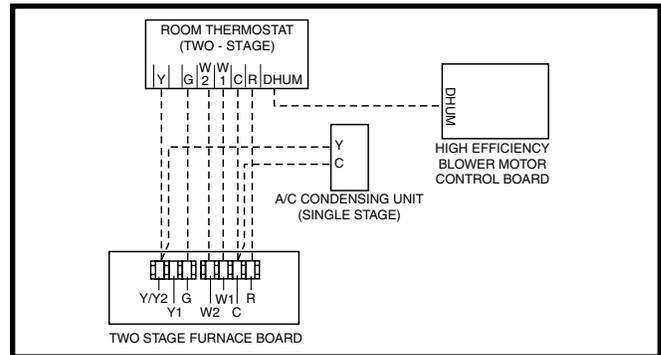
**Figure 21. Wiring Configuration 2**
