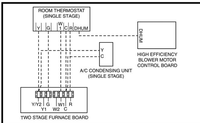
**Figure 20. Wiring Configuration 1**
