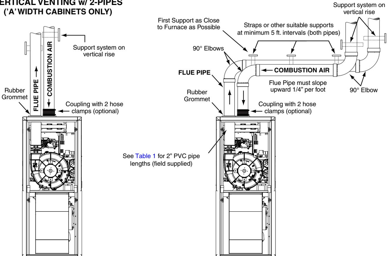
**Figure 32. Horizontal & Vertical Venting (A Width Cabinets)**
