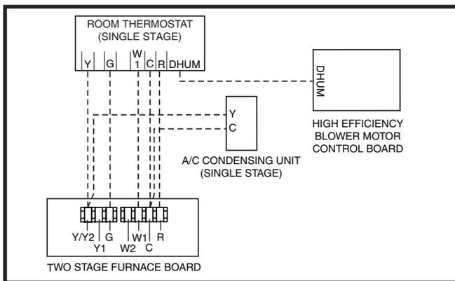
**Figure 20. Wiring Configuration 1**
