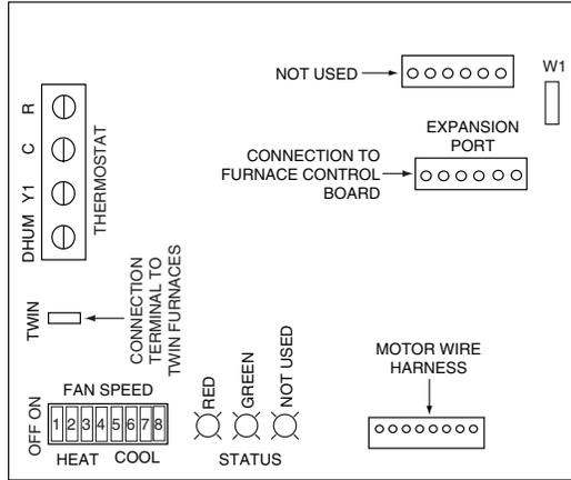
**Figure 27. Two-Stage Fixed Speed Motor Control Board**
