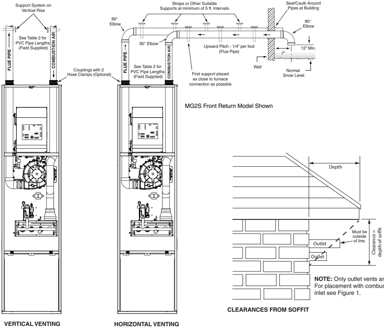
**Figure 29. Horizontal / Vertical Venting & Clearances from Soffit**
