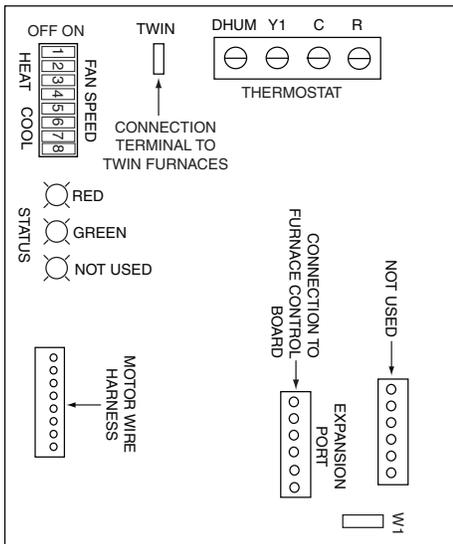
**Figure 26. MG2S Motor Control Board**
