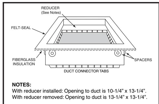
**Figure 8. Duct Connector**
