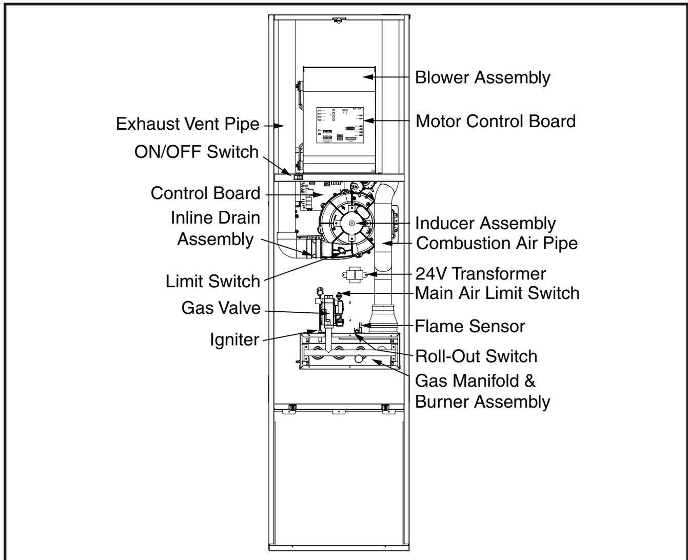
Figure 22. Furnace Components
