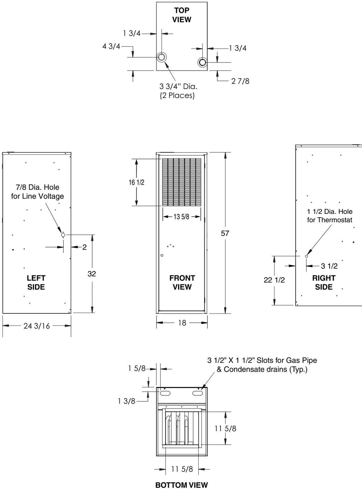
**Figure 18. Furnace Dimensions**
