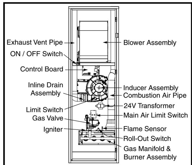
Figure 17. Furnace Components
