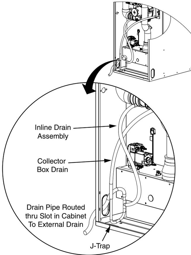
**Figure 11. Condensate Drainage**
