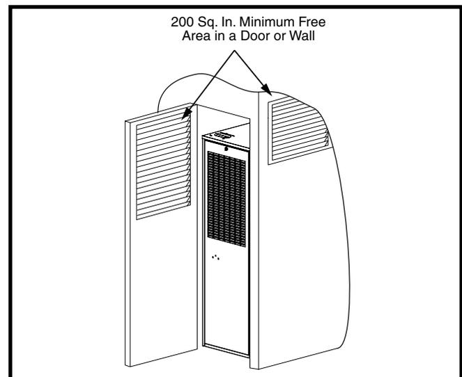
**Figure 6. Closet Installation**
