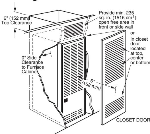
**Figure 2. Closet Installation**
