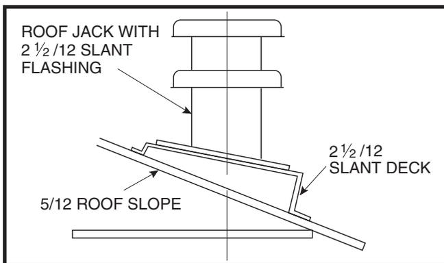
Figure 18. Example of 2 1/2 / 12 Slant Jack with Flashing
