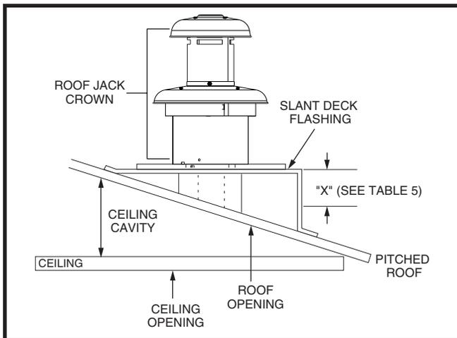
Figure 17. Example of Flat Jack with Flashing
