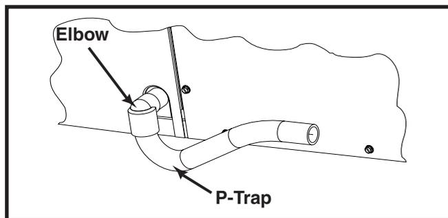
Figure 6. Drain Trap
