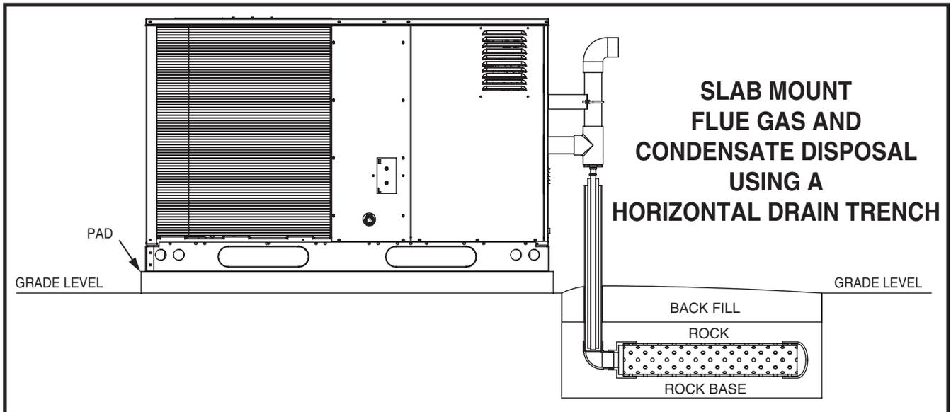
**Figure 22. Condensate Disposal Using A Horizontal Drainage Trench**
