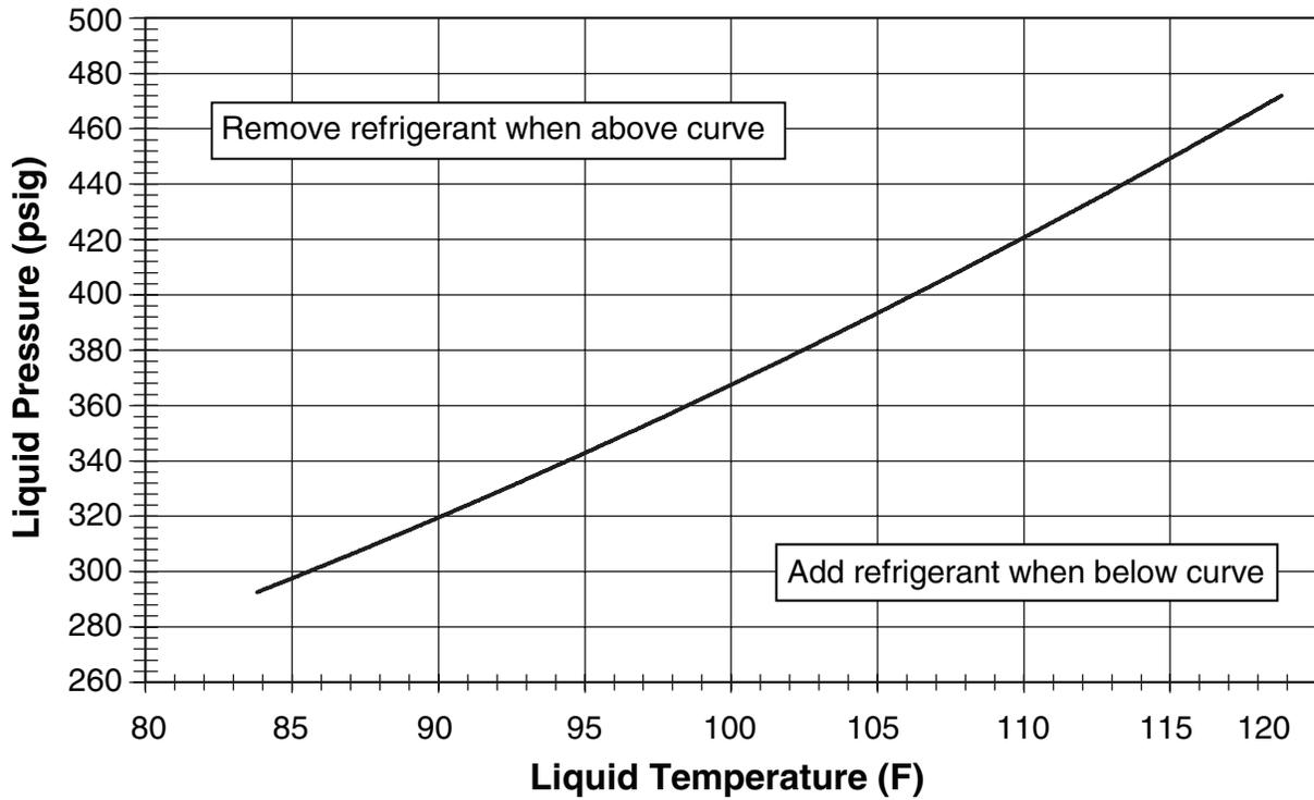
Figure 14. Charging Chart for 2 Ton Units
