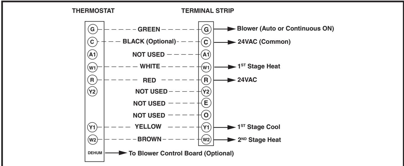
**Figure 10. Two Stage Heating / Single Stage Cooling Configuration**
