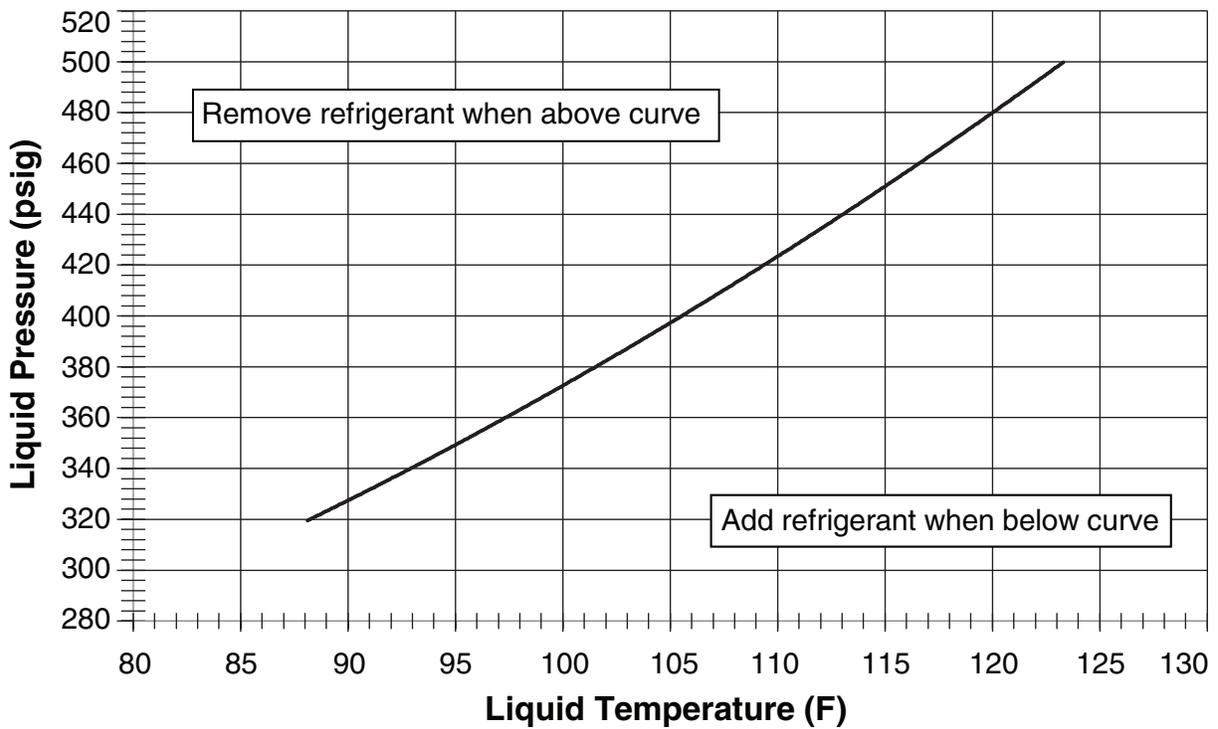
Figure 17. Charging Chart for 3.5 Ton Units
