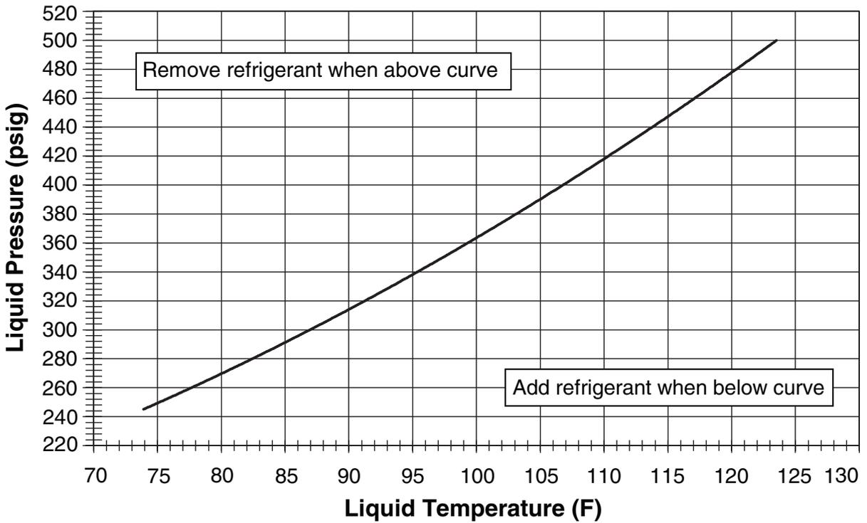
Figure 19. Charging Chart for 5 Ton Units
