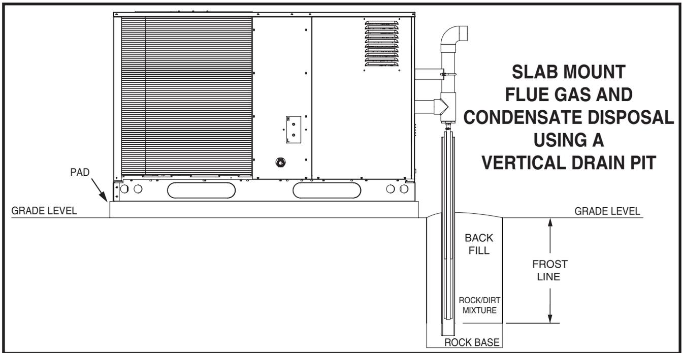
**Figure 21. Condensate Disposal Using A Vertical Drainage Pit**
