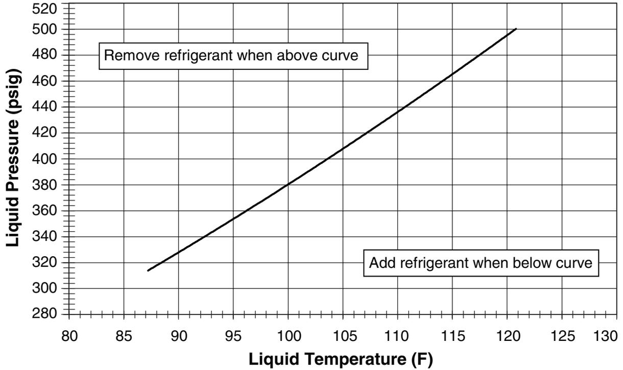
Figure 18. Charging Chart for 4 Ton Units
