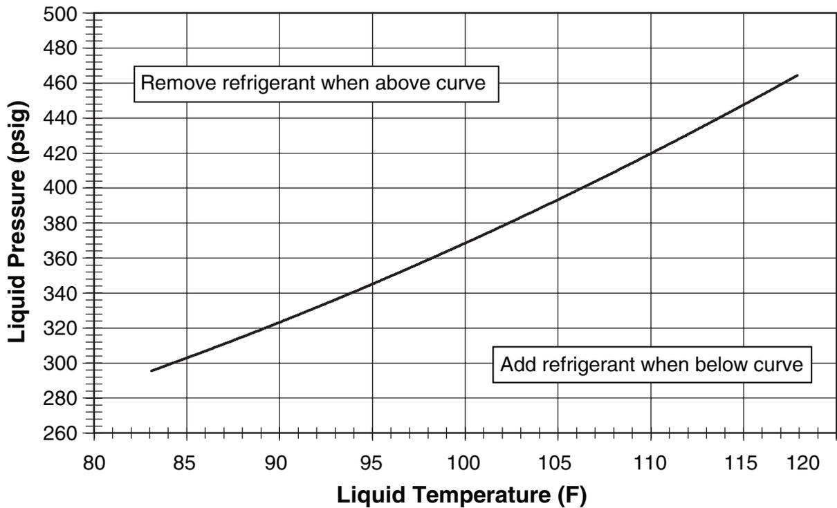
Figure 15. Charging Chart for 2.5 Ton Units
