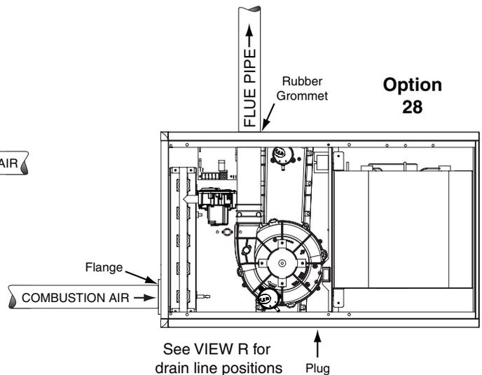
**Figure 45. Venting Options for Horizontal Installations (\*SD Series)**
