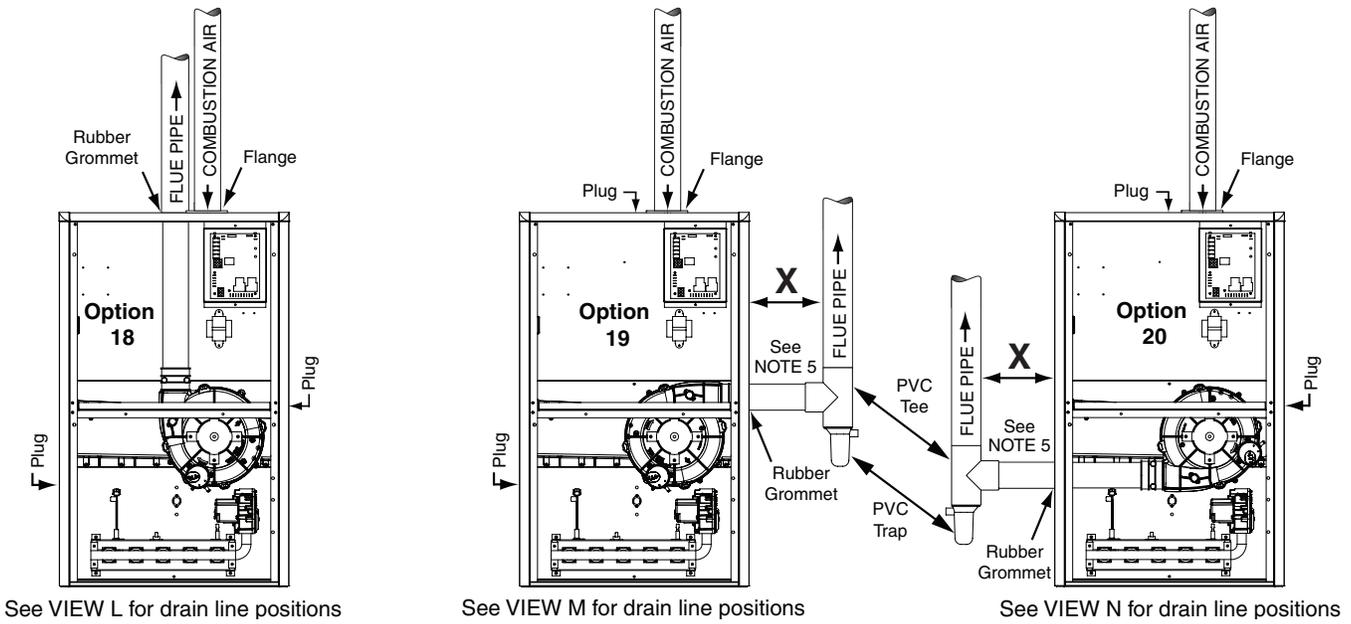
**Figure 42. Venting Options for Downflow Installations (\*SL Series)**
