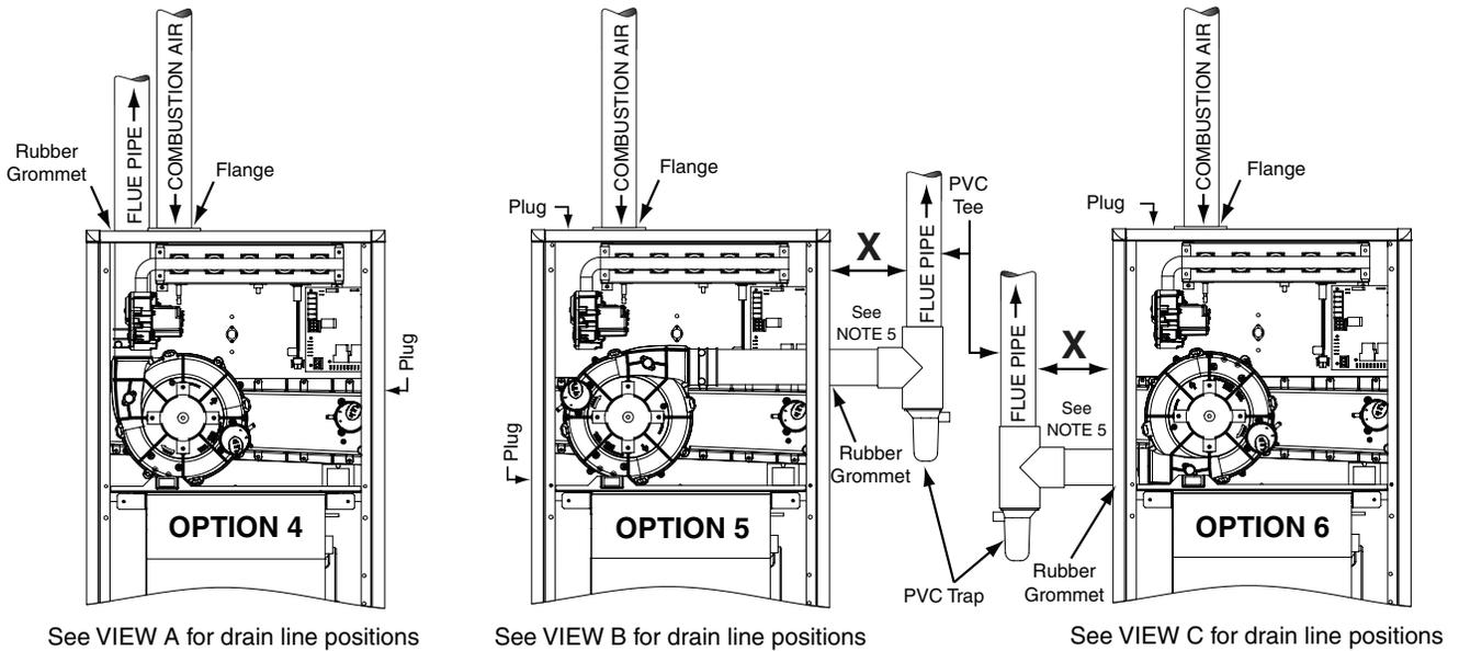
**Figure 39. Venting Options for Upflow Installations (\*SC Series)**
