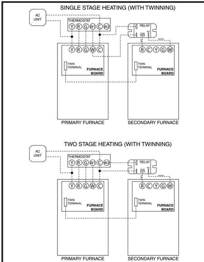
Figure 30. Emerson Single & Two Stage Twinning
