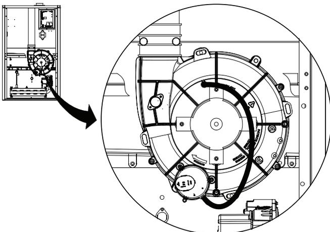
**Figure 16. Pressure Switch Tubing for Downflow Furnaces**
