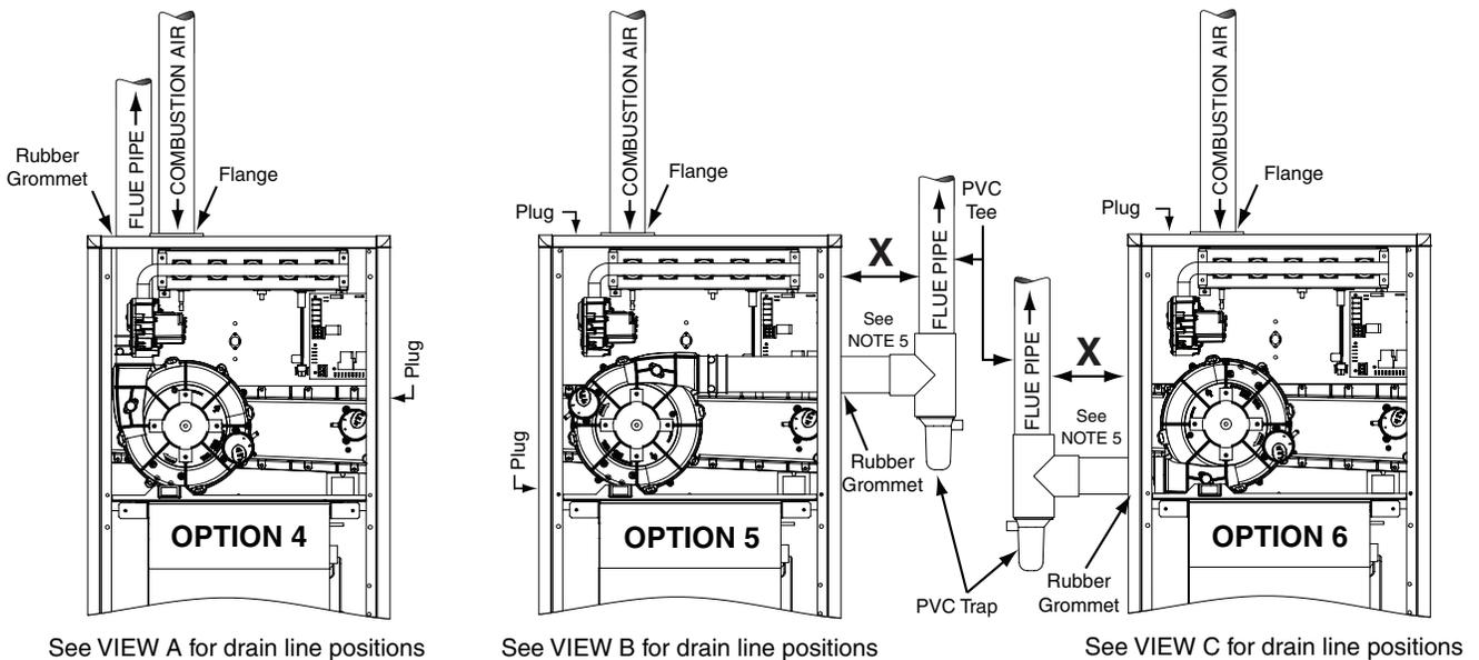
**Figure 36. Venting Options for Upflow Installations (\*SC Series)**
