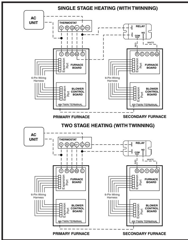
Figure 27. Nordyne/UTEC Single & Two Stage Twinning
