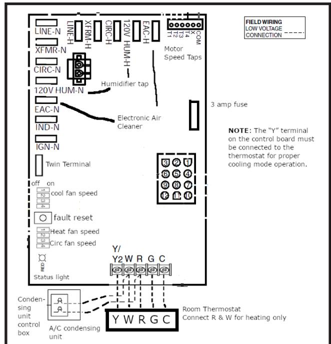
Figure 16. Emerson Low Voltage Field, Four-wire Heating/Cooling Applications
