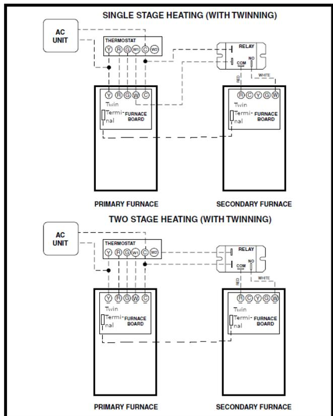
Figure 18. Emerson Single & Two Stage Twinning
