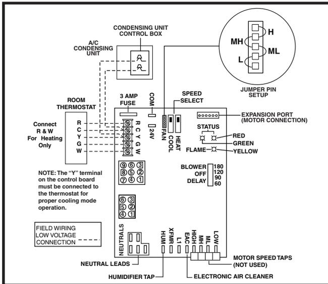
Figure 15. Nordyne/UTEC Low Voltage Field, Four-wire Heating/Cooling Applications
