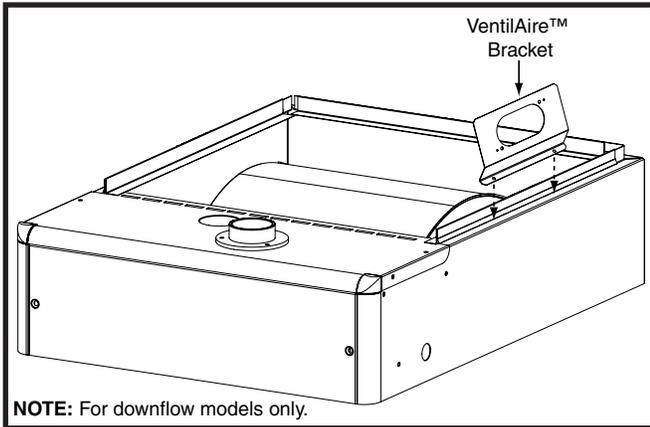
Figure 33. VentilAire™ Bracket
