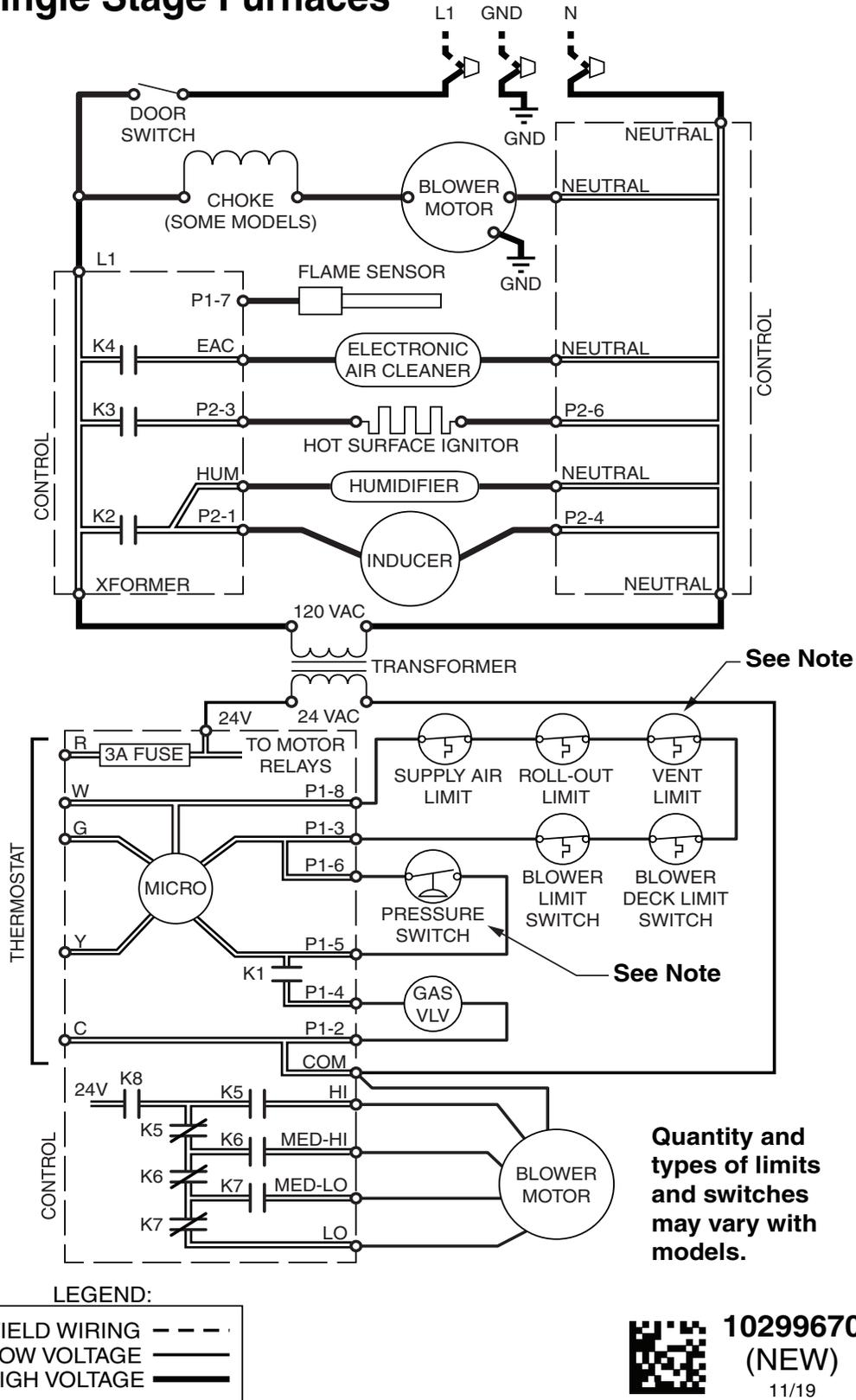
Figure 47. MG3P with Nordyne/UTEC Control Board Ladder Diagram
