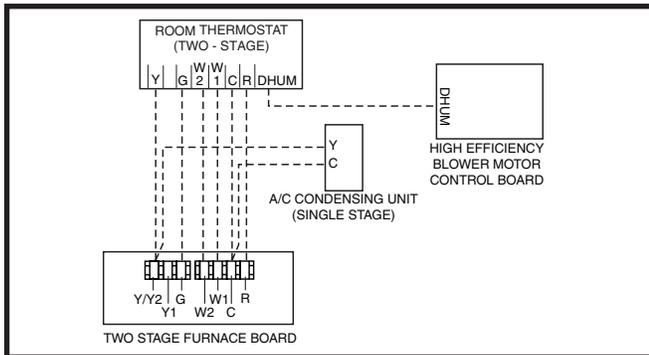
**Figure 39. Wiring Configuration 2**
