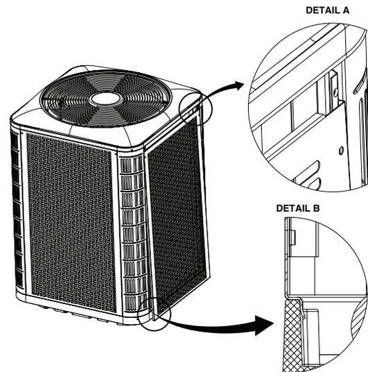
**Figure 4. Panel Installation**
