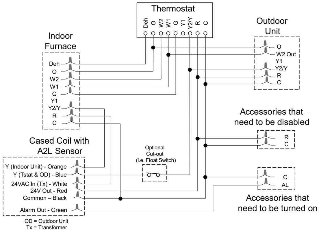
**Figure 8. Typical two-stage furnace with single-stage heat pump.**
