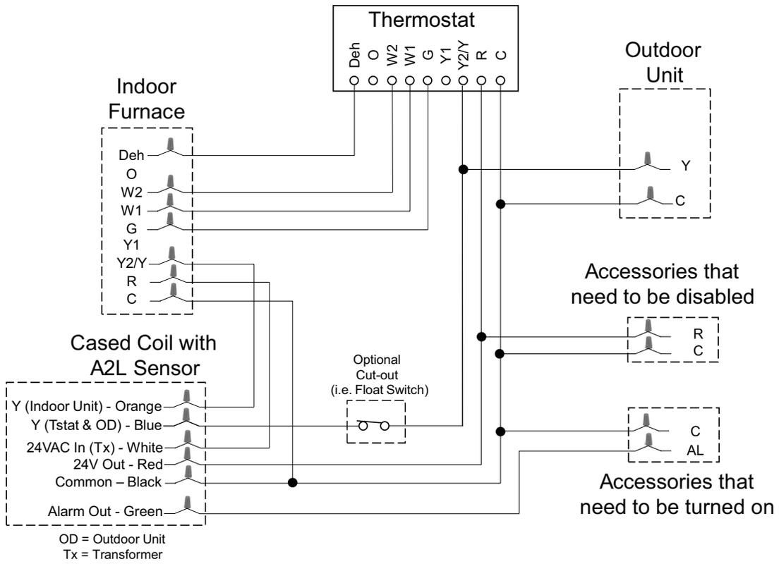
**Figure 11. Typical two-stage furnace with single-stage air conditioner.**
