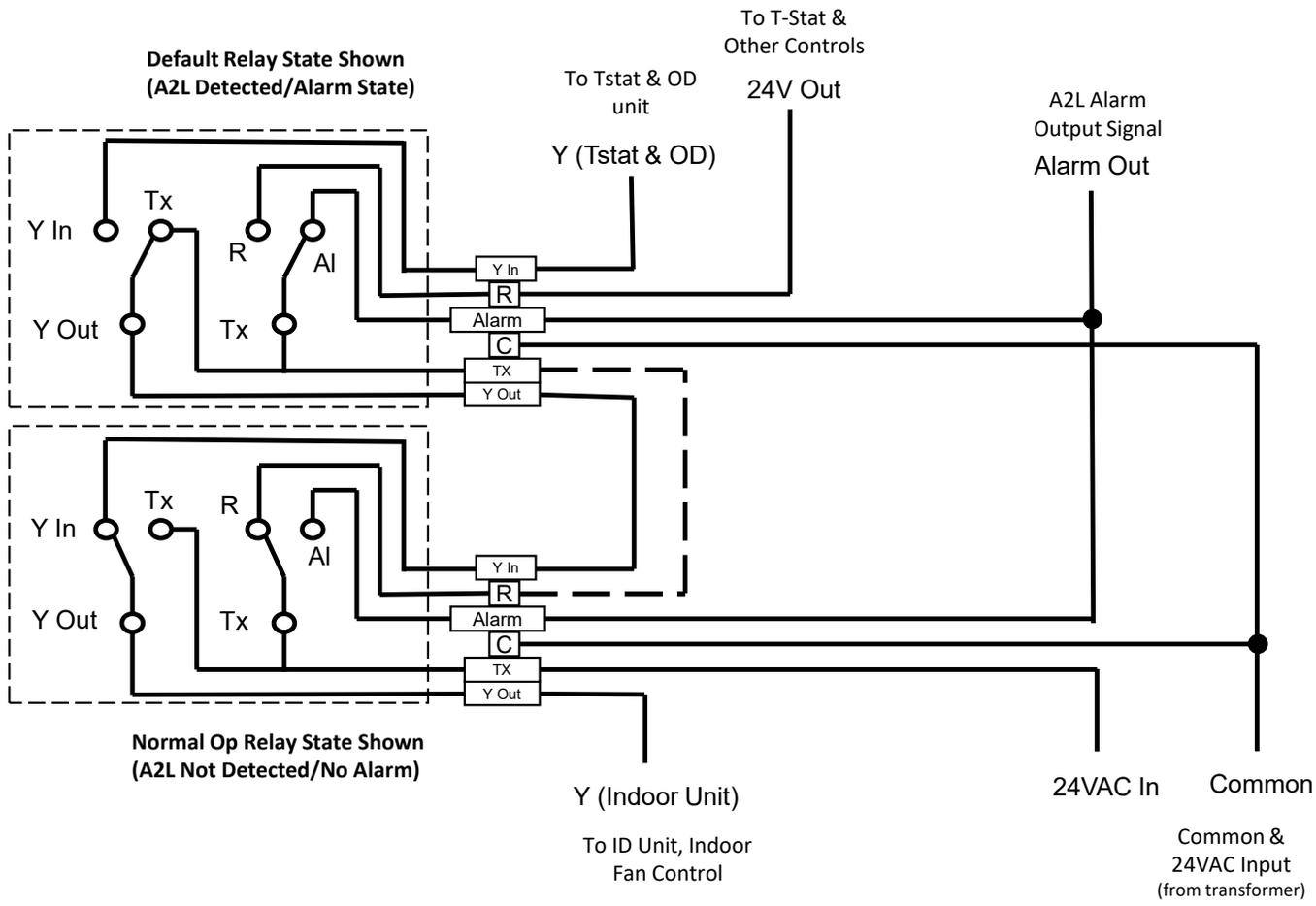
Figure 12. Series Sensor Wiring for systems with 2 or more sensors
