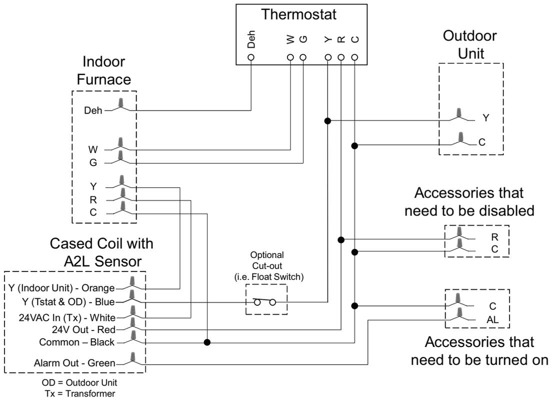
**Figure 10. Typical single-stage furnace with single-stage air conditioner.**
