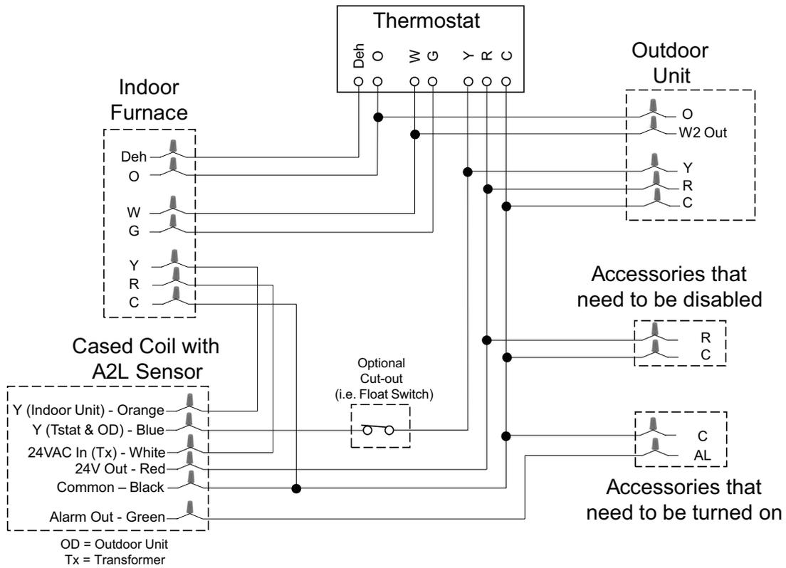
**Figure 9. Typical single-stage furnace with single-stage heat pump.**
