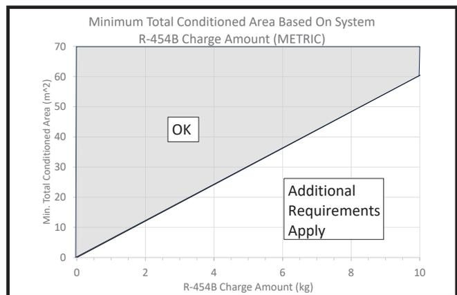
**Figure 4. Minimum Total Conditioned Area Based On R-454B System Charge Amount**
