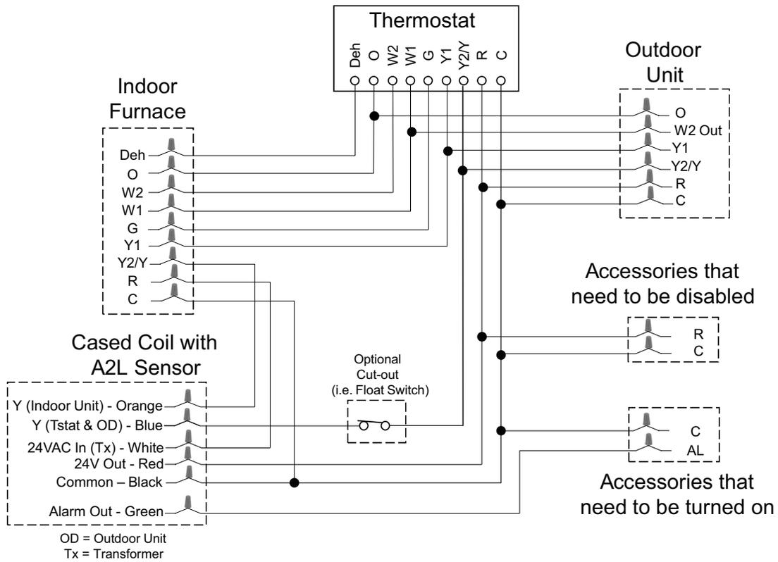
**Figure 7. Typical two-stage furnace with two-stage heat pump.**
