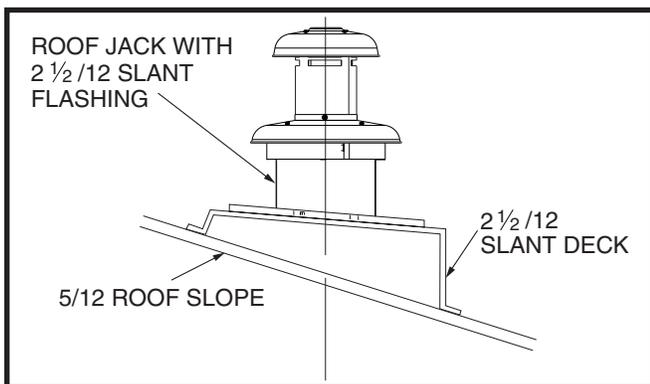
Figure 19. Example of 2 1/2 / 12 Slant Jack with Flashing
