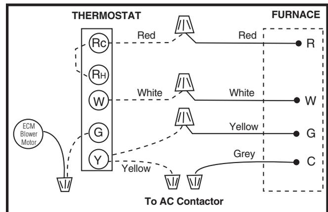
Figure 26. Thermostat Wiring for UTEC/NORDYNE Control boards
