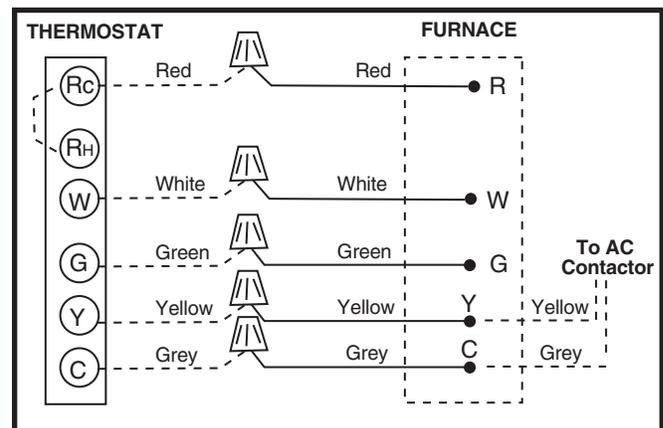
Figure 27. Thermostat Wiring for Emerson/Copeland control boards
