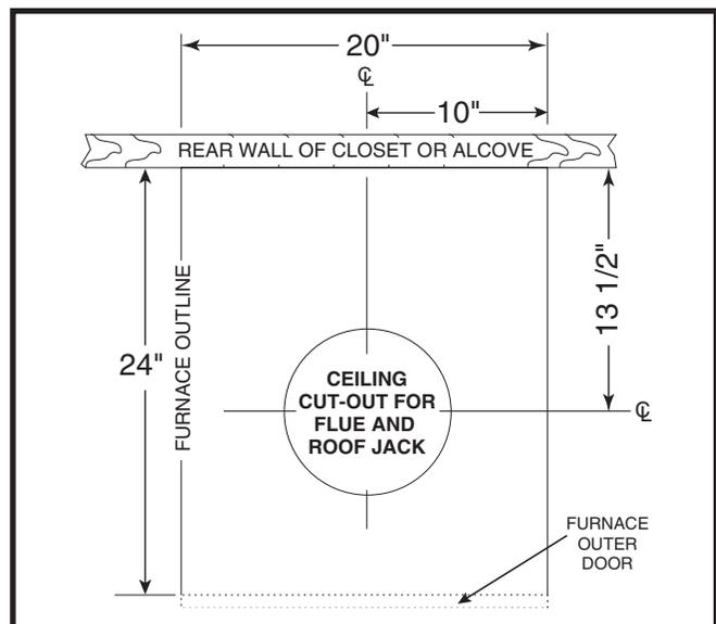
Figure 20. Cut-Out Dimensions for Flue & Roof Jack
