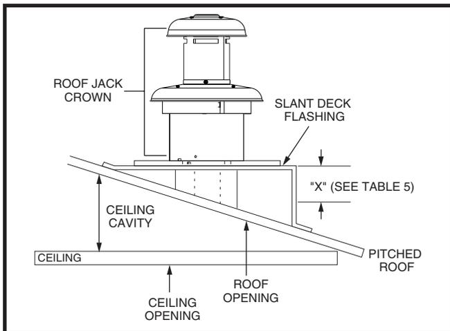
Figure 18. Example of Flat Jack with Flashing
