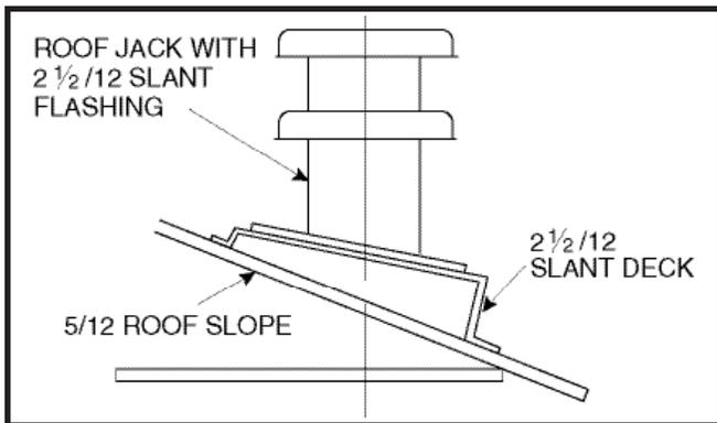
Figure 18. Example of 2 1/2 / 12 Slant Jack with Flashing
