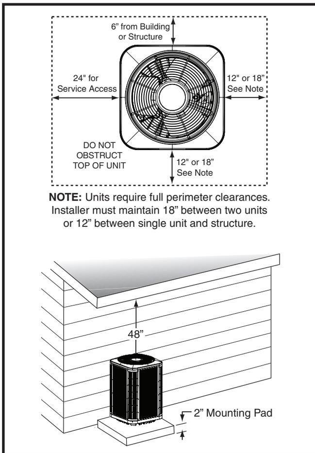
**Figure 1. Clearance Requirements**
