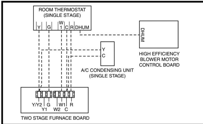
**Figure 20. Wiring Configuration 1**
