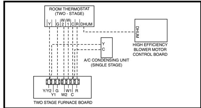
**Figure 21. Wiring Configuration 2**
