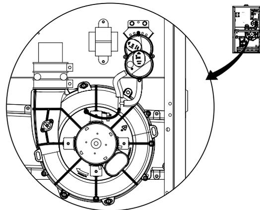
**Figure 13. Pressure Switch Tubing for \*TN Downflow Furnaces**
