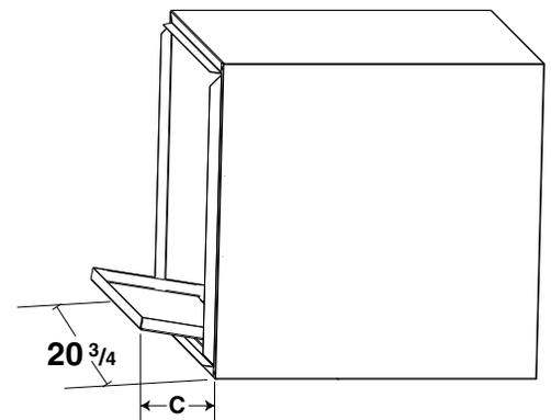
Figure 2. Horizontal Left Configuration with Drain Pan Extension
