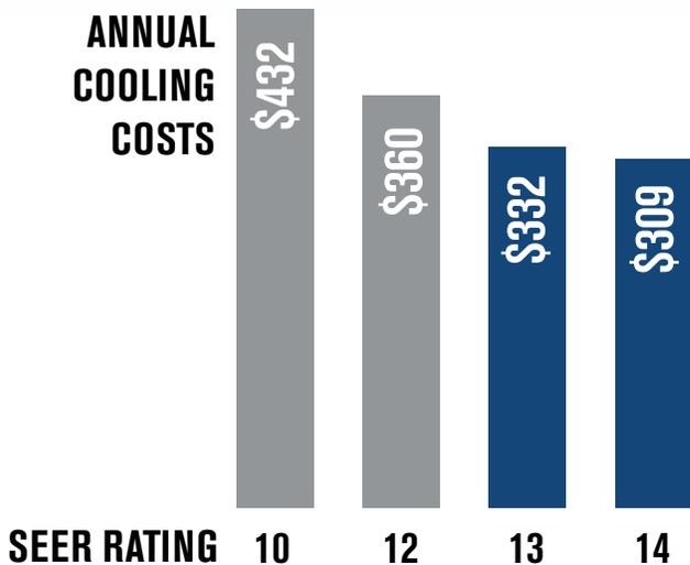
Annual costs based on 36,000 Btu unit, 1,500 cooling load hours and .08/kwh. Actual costs may vary depending on climate conditions, energy rates and patterns of usage.
