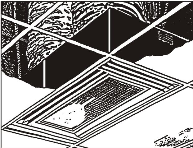
2. Connect duct to the diffuser assembly and slide the diffuser and duct into framed opening and secure with screws. In applications where long duct drops are required, it is advisable to connect a wire to duct to pull it up to the roof curb.
