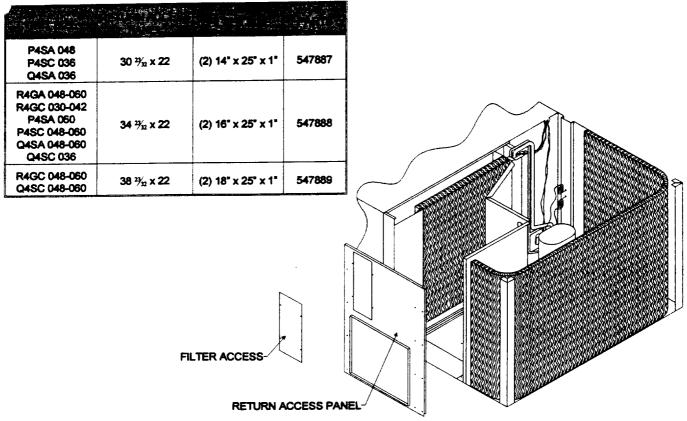
STEP 4: Put in place and secure new return access panel.
