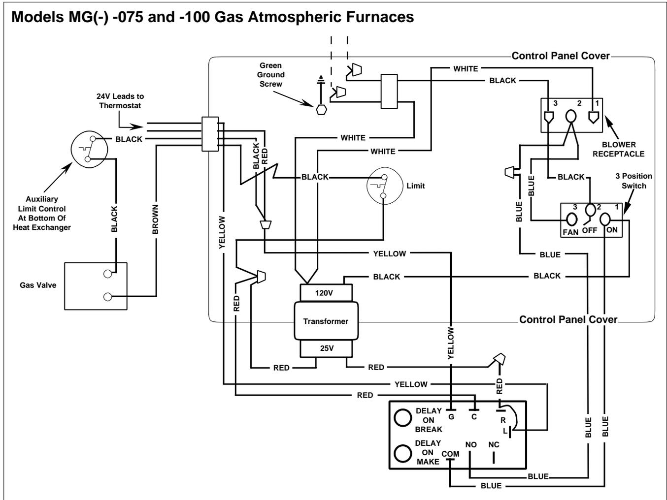
Figure 2. MGH Furnace Wiring Diagram
