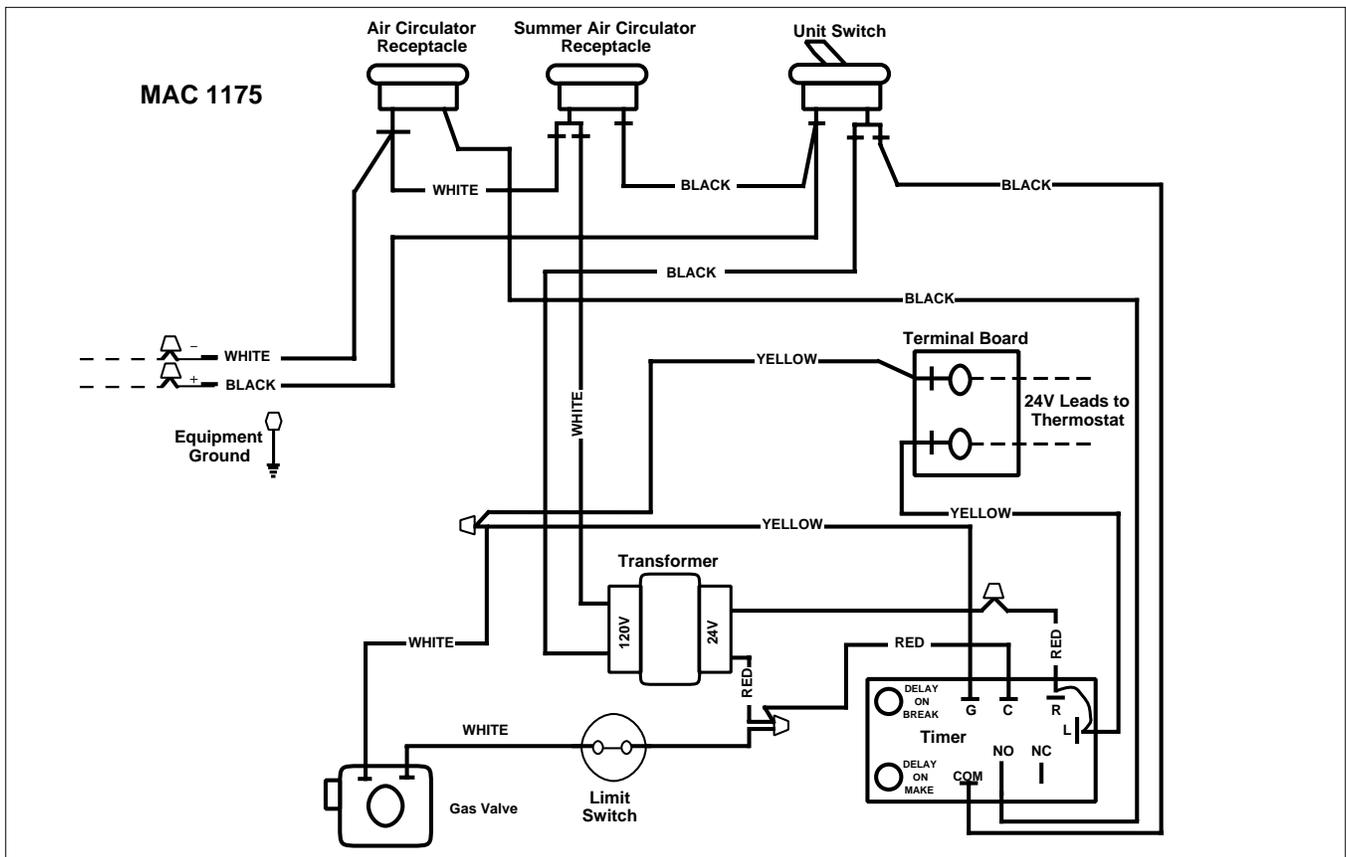
Figure 1. MAC 1175 Wiring Diagram
