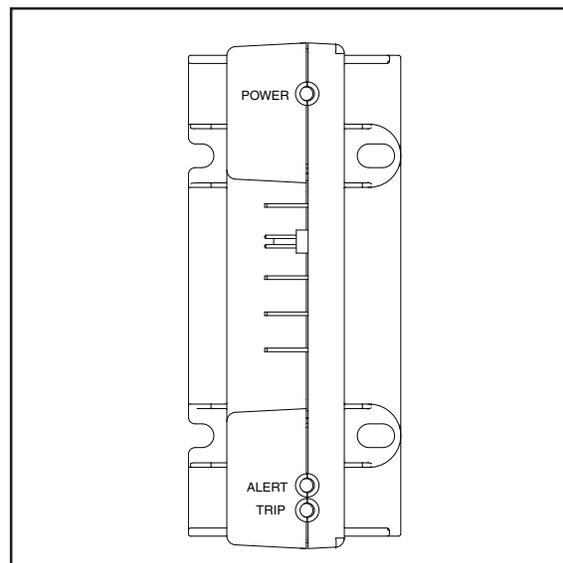
**Figure 2. Comfort Alert™ Diagnostics Module**
