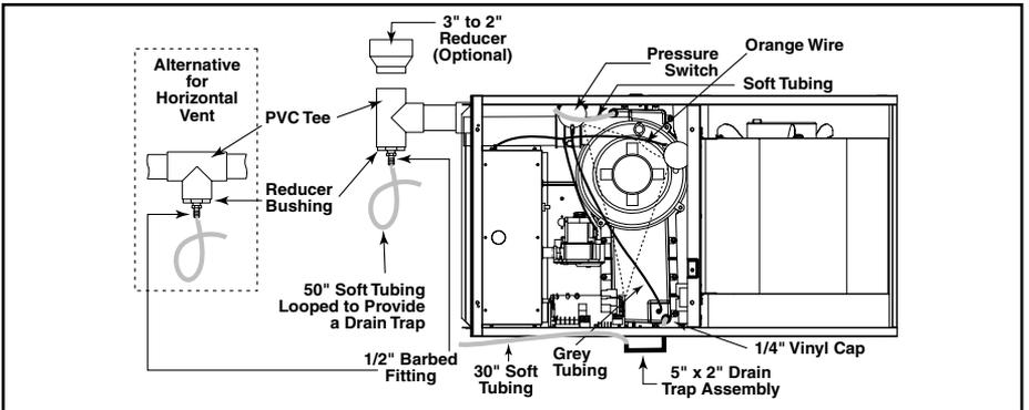
**Figure 4. 90+ Upflow Converted for Horizontal Installation (Horizontal Left)**
