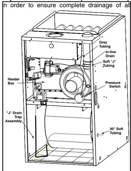
**Figure 2. 90+ Upflow Furnace as Shipped From the Factory**
