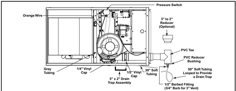
**Figure 3. 90+ Upflow Converted for Horizontal Installation (Horizontal Right)**
