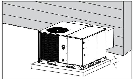
**Figure 6. Ground Level Installation**
