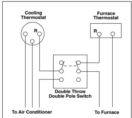
Figure 2. Thermostat Interlock System
