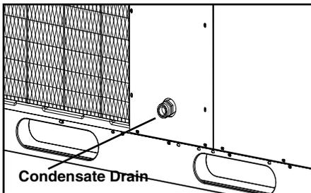
**Figure 5. Condensate Drain**
