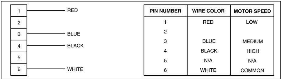
**Figure 9. Motor Lead Connector**
