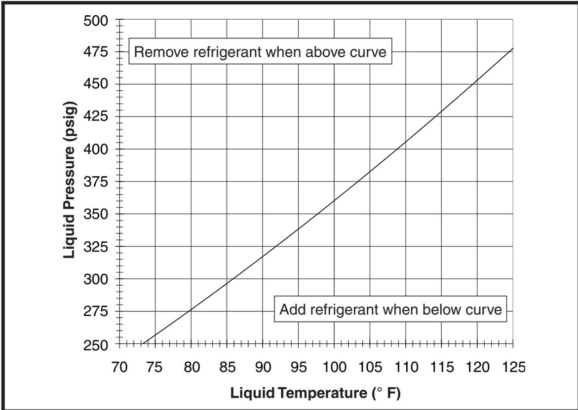
Figure 6. Charging Chart for 4 Ton Units
