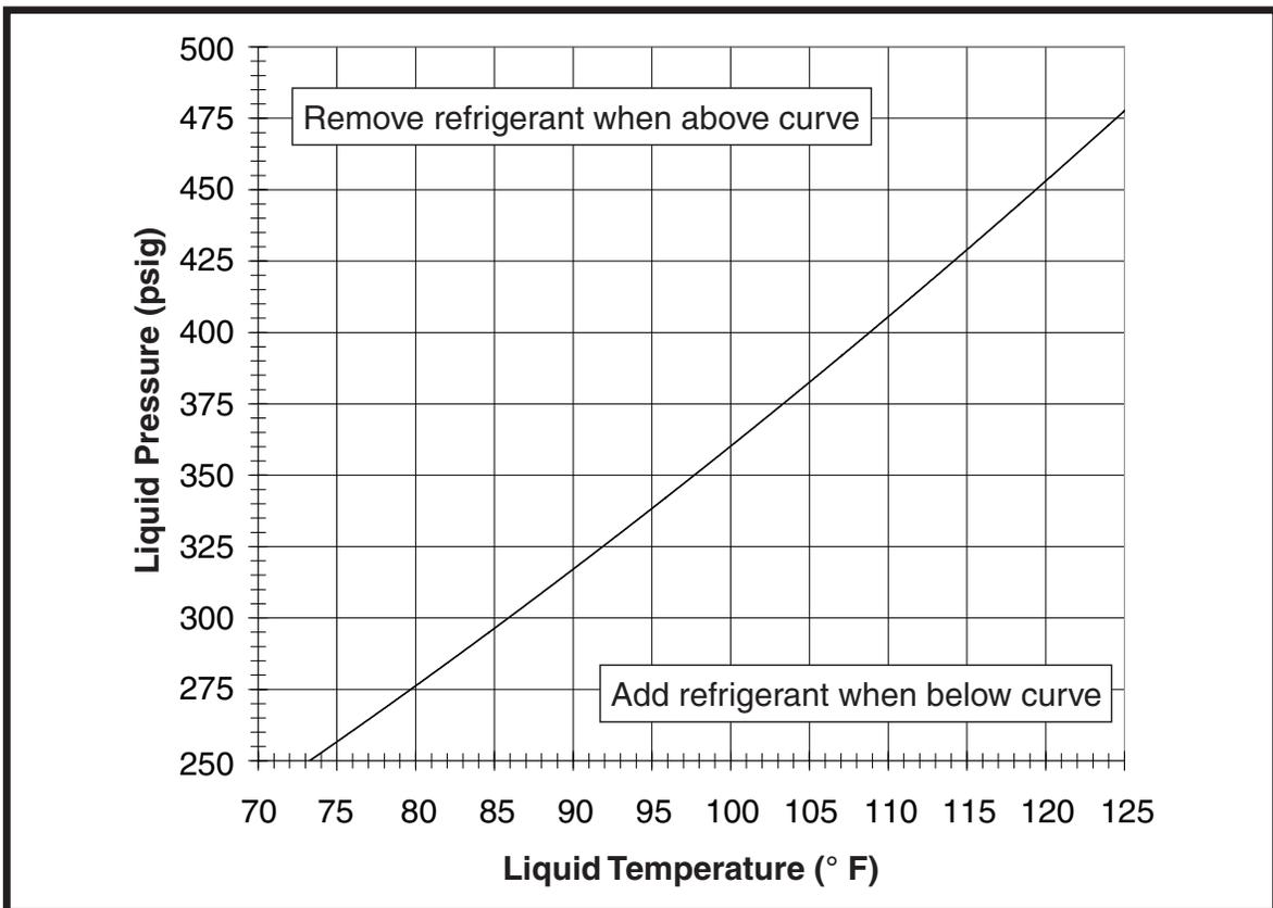
Figure 7. Charging Chart for 5 Ton Units
