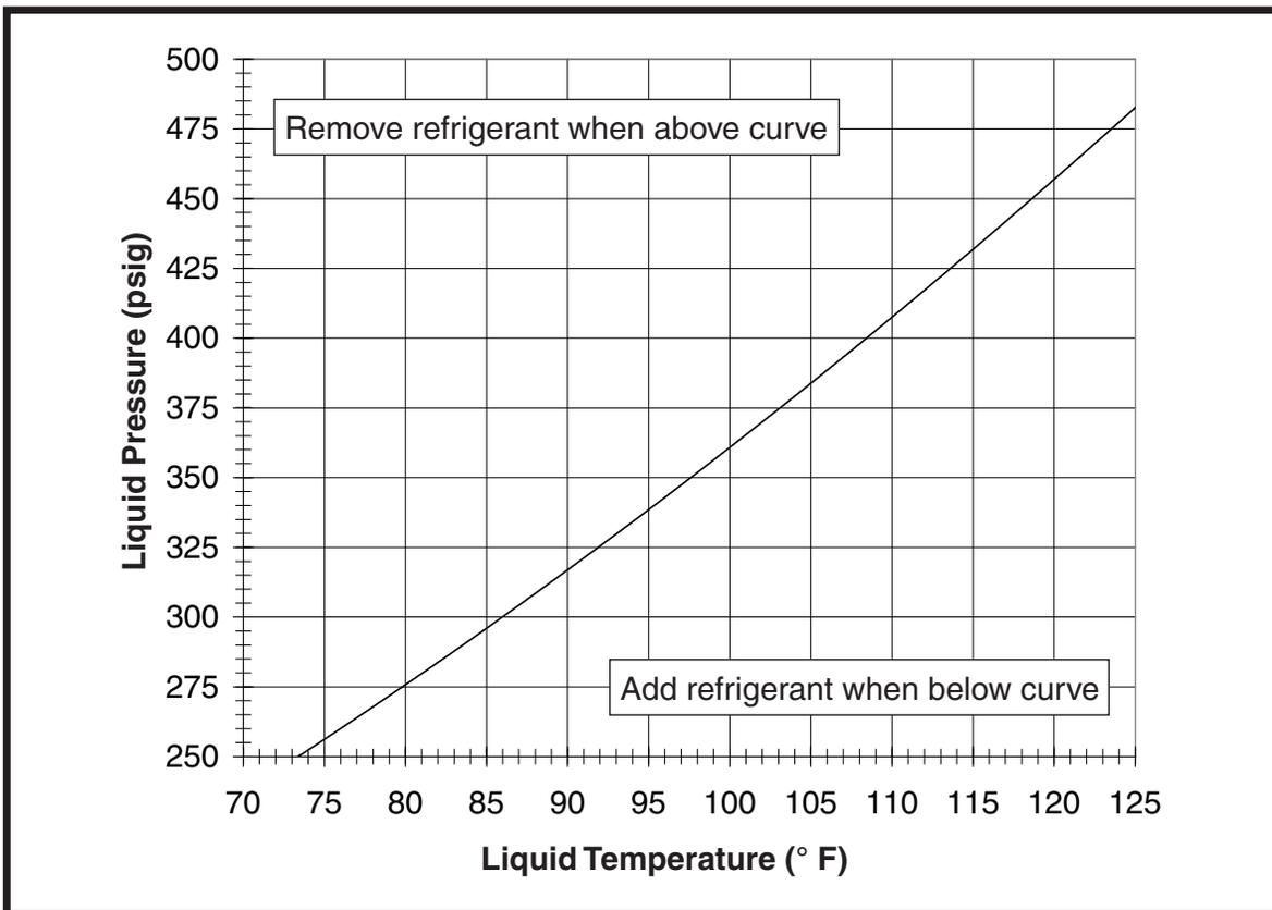
Figure 5. Charging Chart for 3 Ton Units
