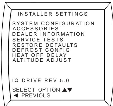
Other than in the splash screen displayed when power is first applied to the controller, this is the only screen which displays the controller software version number.
