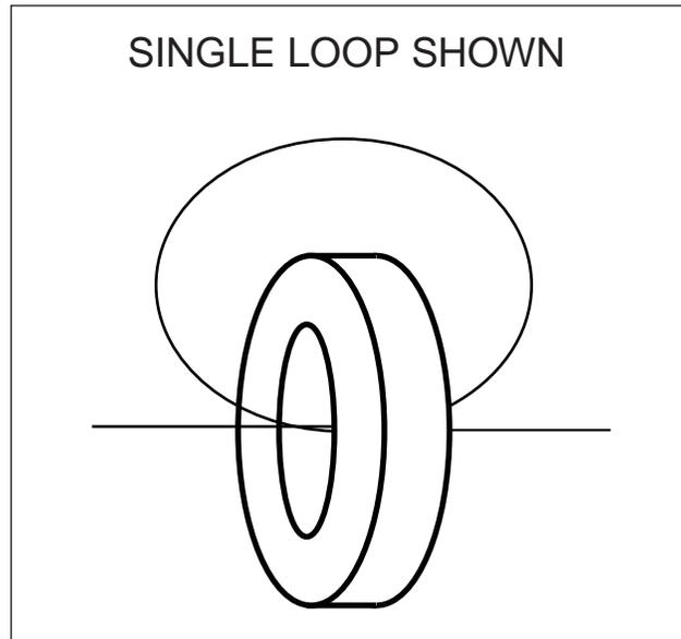
Figure 7. Wire Looping Through a Toroidal Choke
