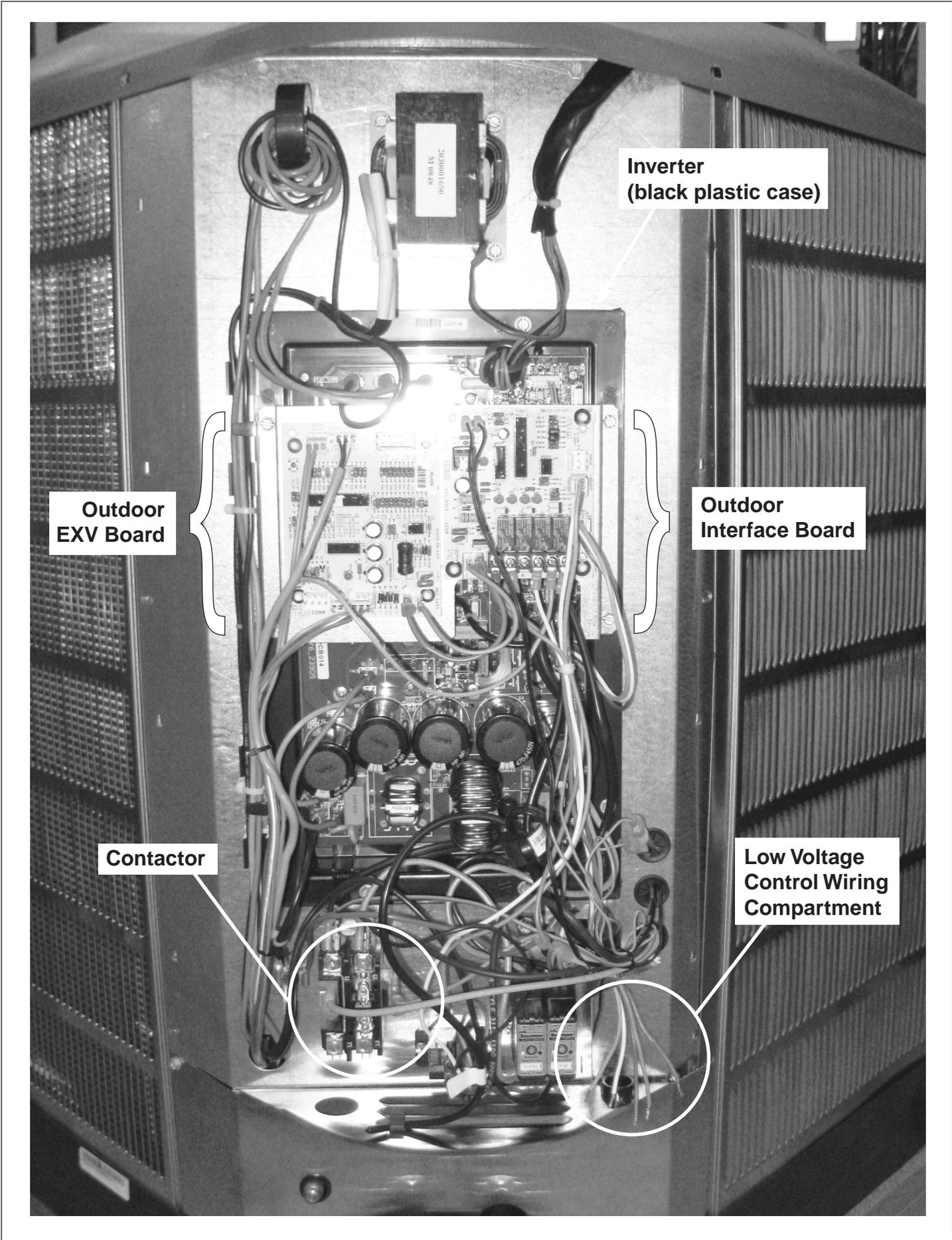
Figure 3. iQ Drive Heat Pump Control Panel
