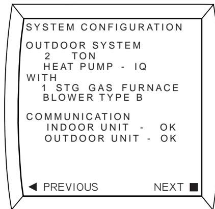
The words under OUTDOOR SYSTEM and WITH describe the system components as automatically detected by the controller. Both entries under COMMUNICATION should show “OK”. If “CHECK” appears, it is an indication that either communication wiring is incomplete or incorrect, or the outdoor unit is not powered up. Proceed through subsequent screens by using either the ▶ or ■ key (indicated by “NEXT”).
