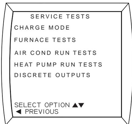
**NOTE:** While running the system from Service Tests is convenient for some startup operations, much of the normal fault handling and diagnostic message functionality is disabled.
