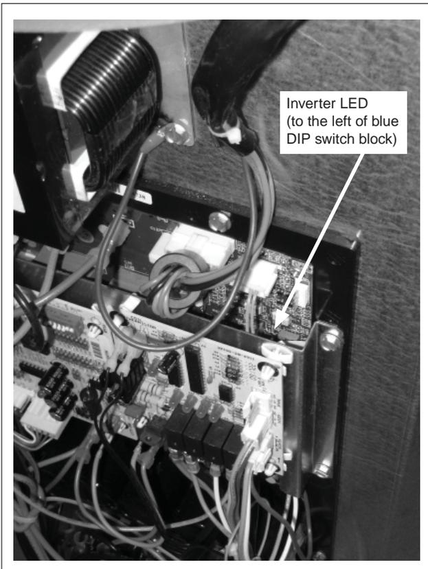
Figure 12. Inverter LED Location
