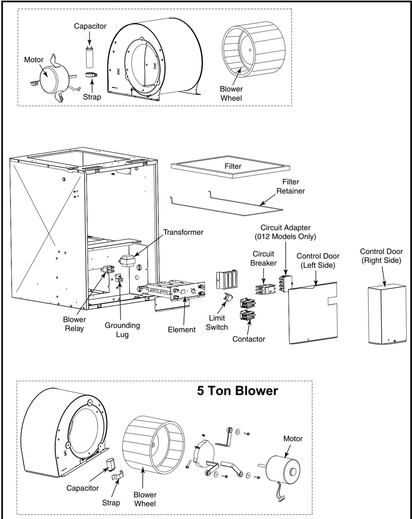
**Figure 19. E3 Furnace Components**
