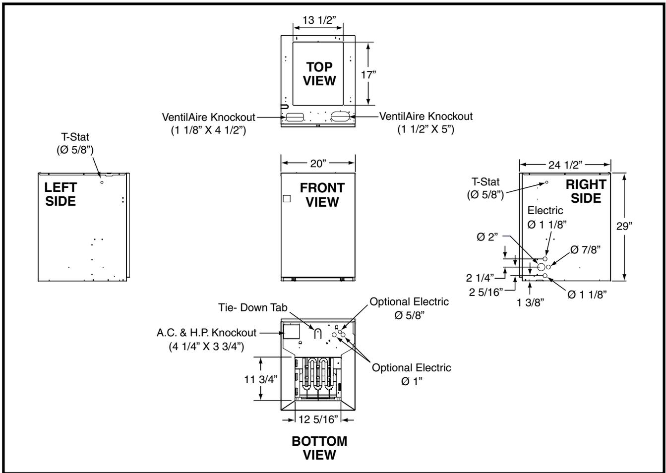
Figure 20. E3 Furnace Physical Dimensions
