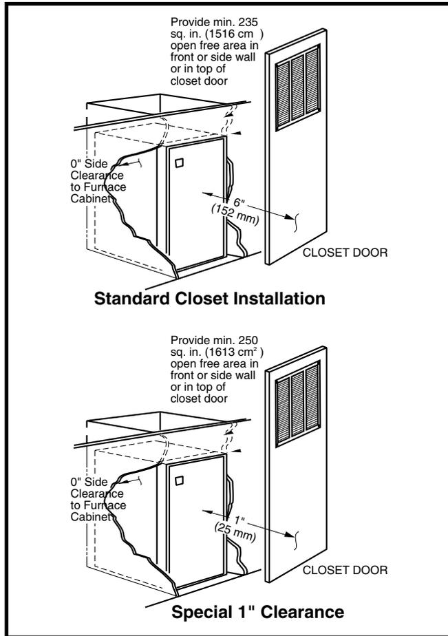
Figure 14. Closet Installation
