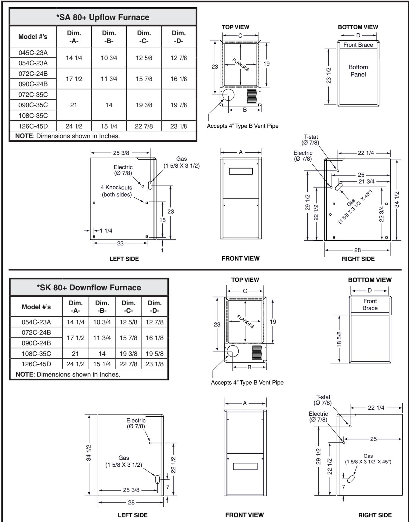
**Figure 18. Furnace Dimensions**
