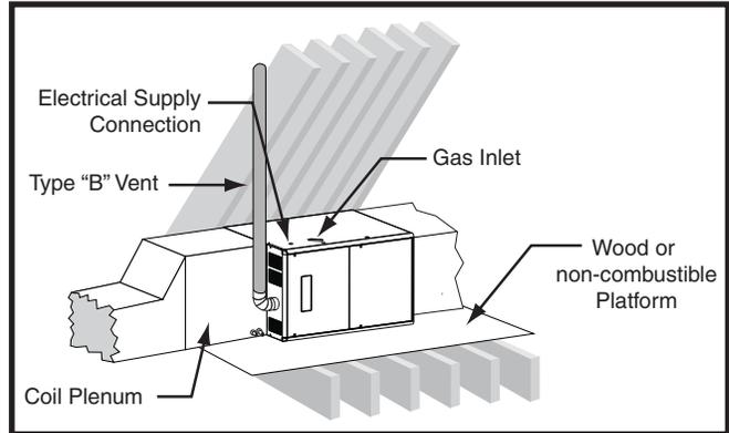
**Figure 8. \*SA Horizontal Installation on a Platform**
