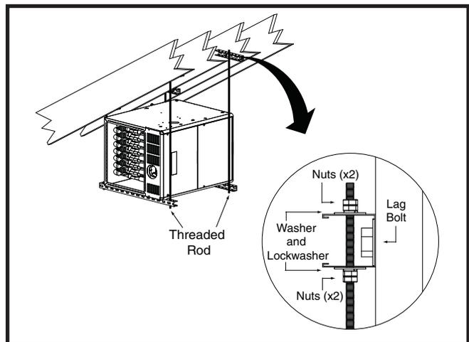
**Figure 9. \*SA Horizontally Suspended in Attic**
