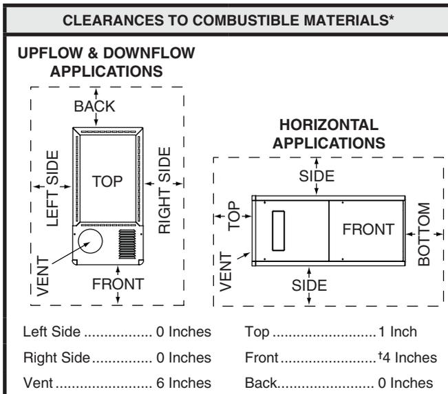
\*Allow 24 in. minimum clearance for servicing. Recommended clearance is 36 in.
