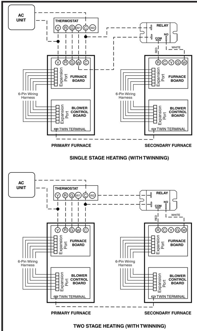
Figure 16. Single Stage Twinning
