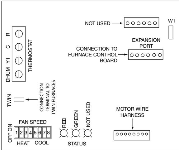
**Figure 22. Two-Stage Fixed Speed Motor Control Board**
