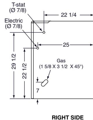
**Figure 21. Furnace Dimensions**
