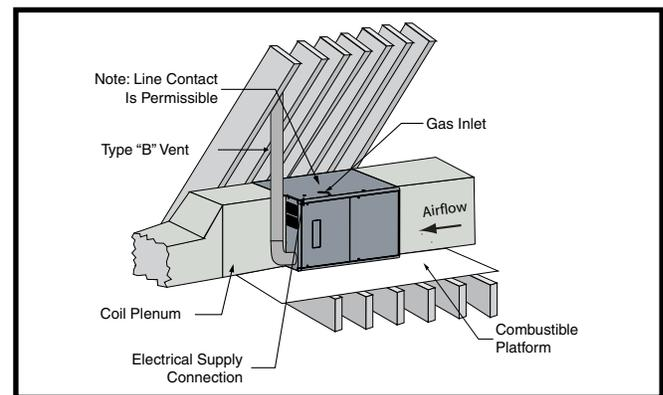
**Figure 7. \*TA Horizontally Installed on a Platform**
