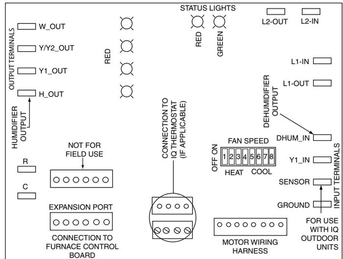
**Figure 23. Two-Stage Variable Speed Motor Control Board**
